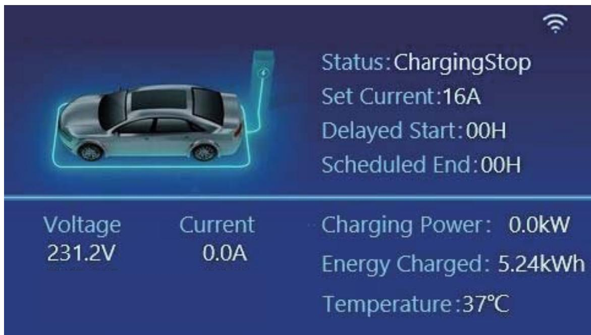
In the charging state, by manually swiping the card to stop charging, the device stops charging. The display effect is shown in the above figure.
