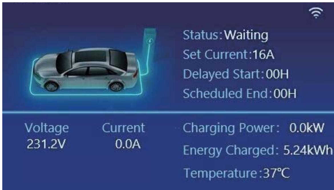
When the vehicle is fully charged, it will automatically stop charging or the user has set a delayed charging time, and the device is waiting to start charging. The display effect is shown in the above figure.
