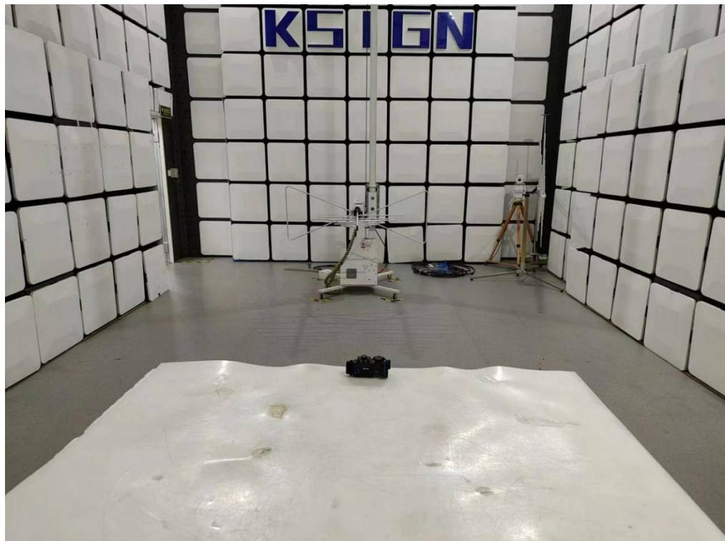
Emissions in frequency bands (below 1GHz)
