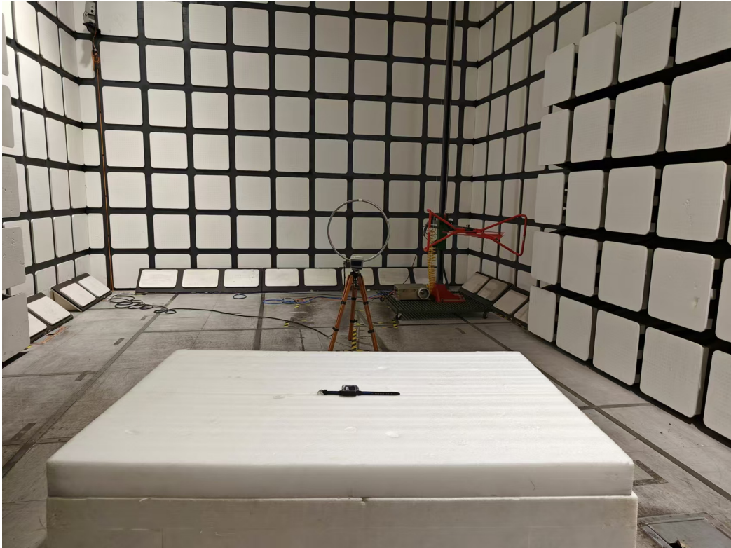
Radiated Emissions View (Below 30MHz)
