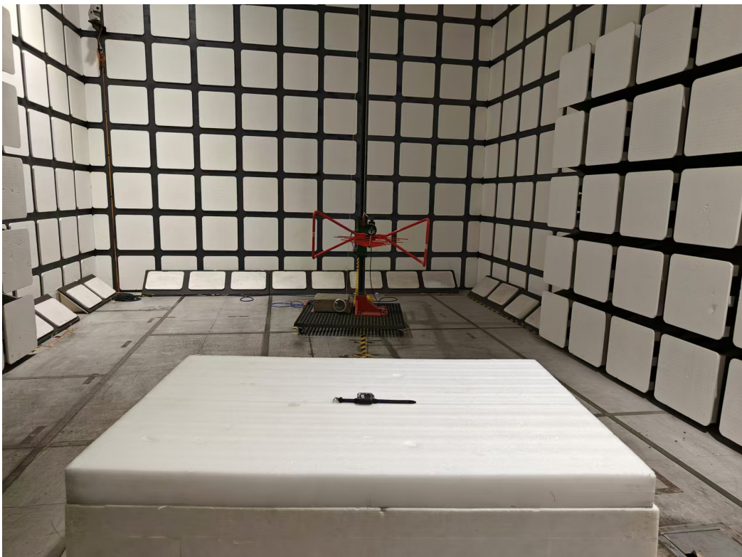
Radiated Emissions View (Below 1 GHz)
