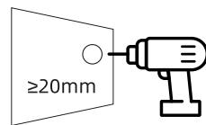
B: Choose the best location on the wall (near the end of the power cord) and drill a hole at least 20 mm in diameter to ensure that the power cord can pass through this hole.
