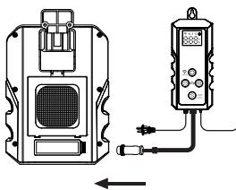
D: Installation of the controller power cord: connect the power cord with the host power hole, and then tighten the nut on the power cord clockwise.
