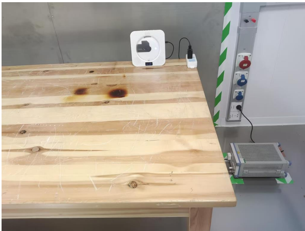
Power Line Conducted Emission
