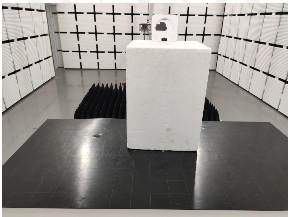
Spurious Radiation Emissions Test (>1G)
