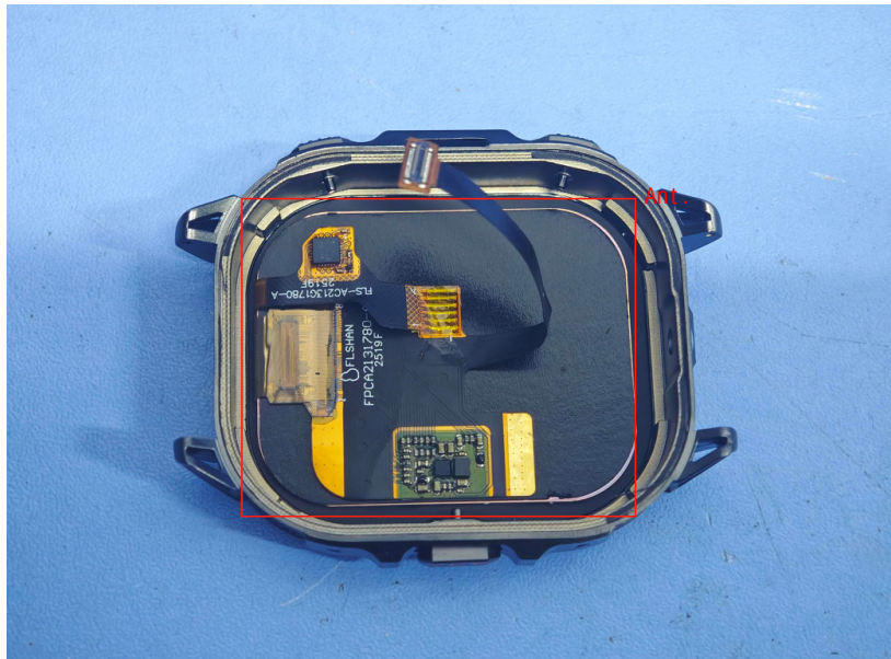
The watch casing is the antenna.
