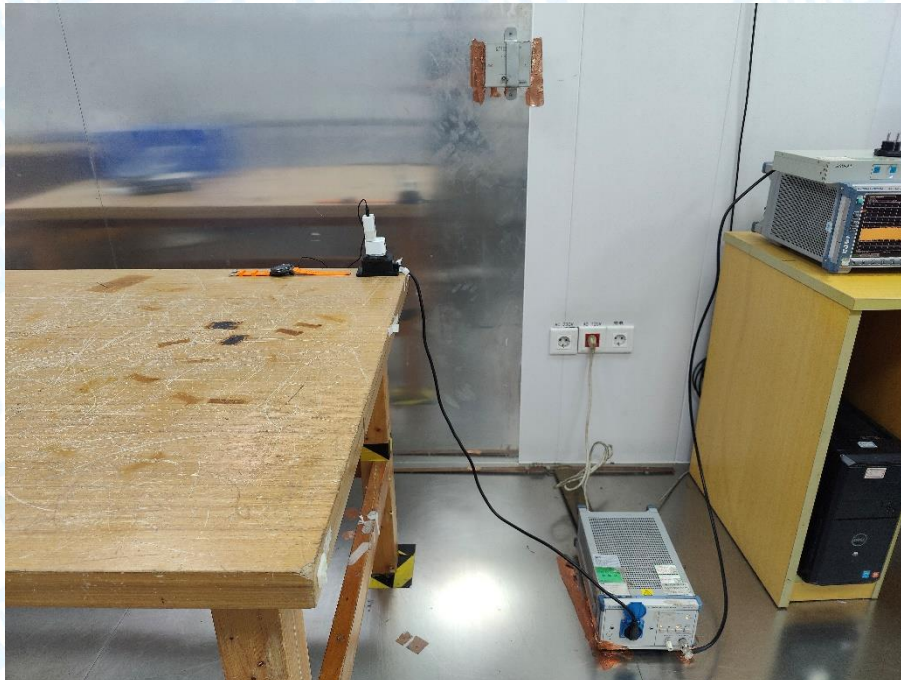
Photo of Setup for Radiated Emission (30MHz~1GHz)
