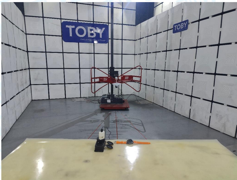
Photo of Setup for Radiated Emission (30MHz~1GHz)
