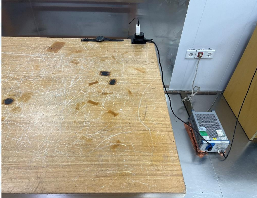
Photo of Setup for Radiated Emission (30MHz~1GHz)
