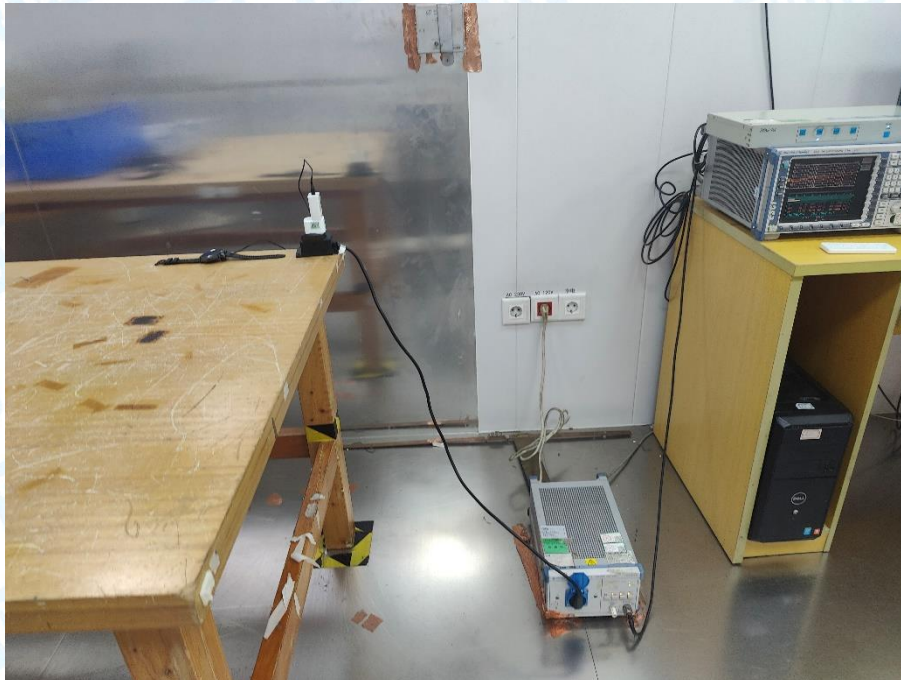
Photo of Setup for Radiated Emission (30MHz~1GHz)
