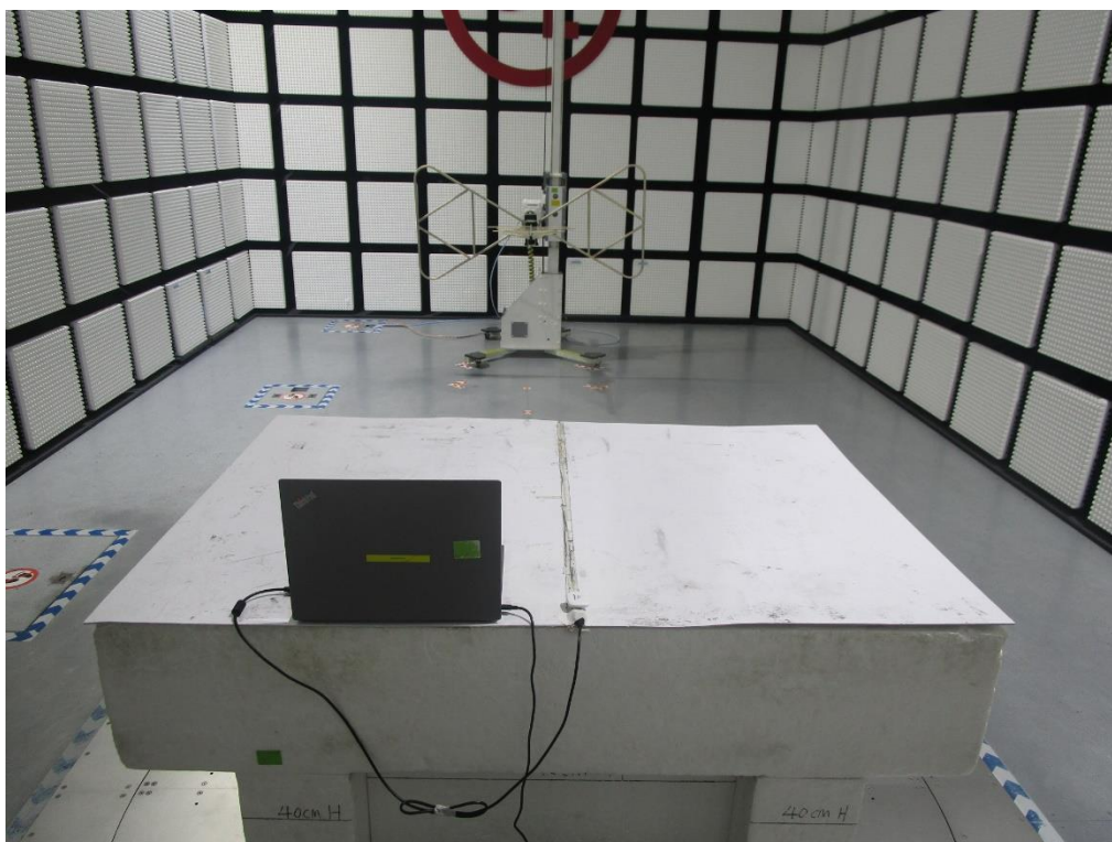
Radiated Band edge and Spurious Emission Below 1GHz
