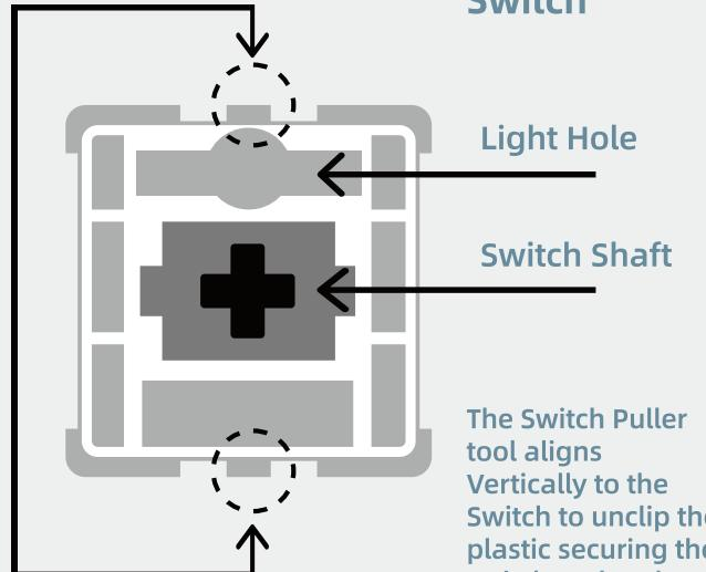
The Switch Puller tool aligns vertically to the Switch to unclip the plastic securing the switch to the plate.
