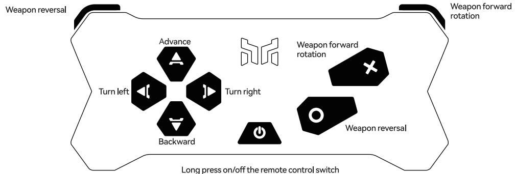
**Tip:** If your combat robot is walking backwards, you can press and hold the up and down buttons on the remote control for 5 seconds to modify the direction of the machine's movement
