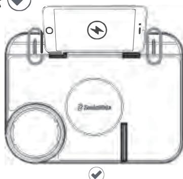
When using the front/side wireless charging function, please place the phone in the effective charging area (the area protected by the Baffle).
