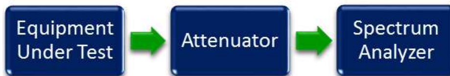
Figure 5. Conducted Spurious Emissions Test Setup
