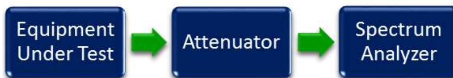
Figure 7. Band Edge Test Setup
