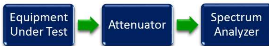
Figure 7. Band Edge Test Setup
