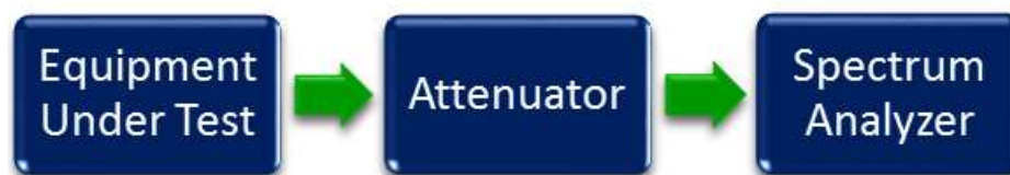
Figure 3. Occupied Bandwidth Test Setup
