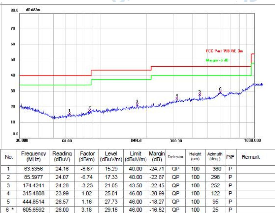
1. Margin = Measurement Level - Limit ; Measurement Level=Test receiver reading + correction factor
