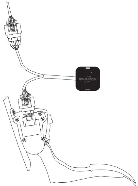
④ Start the car. The LED light on the shell will turn on (it will automatically turn off after one minute), indicating that the installation is correct.
