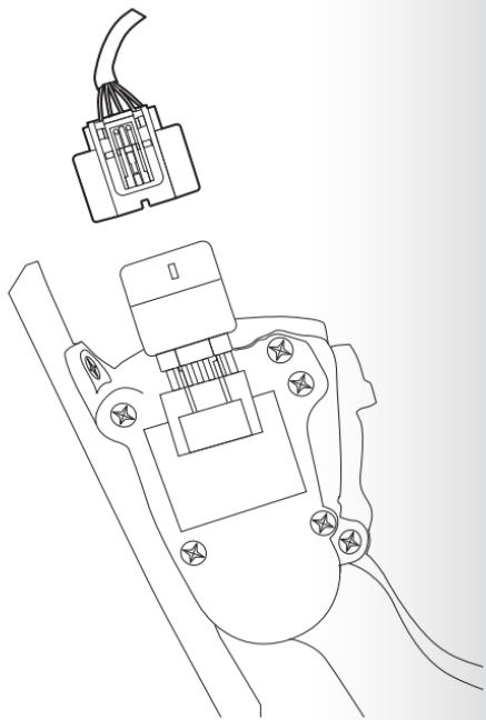
③ Connect the female port of the Roar Pedal wiring to the pedal port and connect the male port to the original sensor harness. (Pay attention to the installation direction and ensure it is installed correctly.) The installation is complete, as shown in the figure below:
