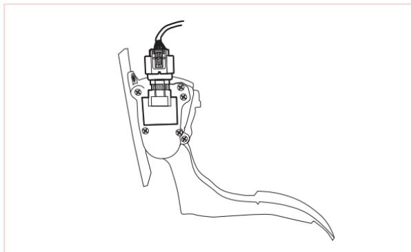
② Unplug the original sensor harness from the accelerator pedal as shown below: (Note that most of them are locked. Press down the lock clip on the female port and easily pull it out)
