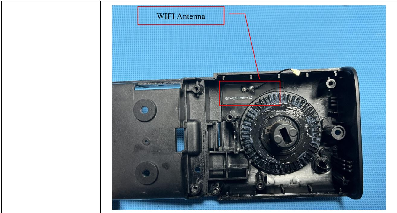
NOTE: Solder Board-Component View 3 and View 7 the antenna in the picture has been shielded and has no transmitting function.
