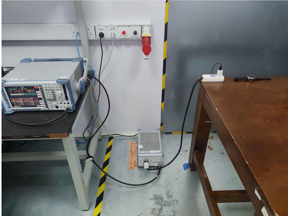
Conducted emissions at AC power line (150kHz-30MHz)
