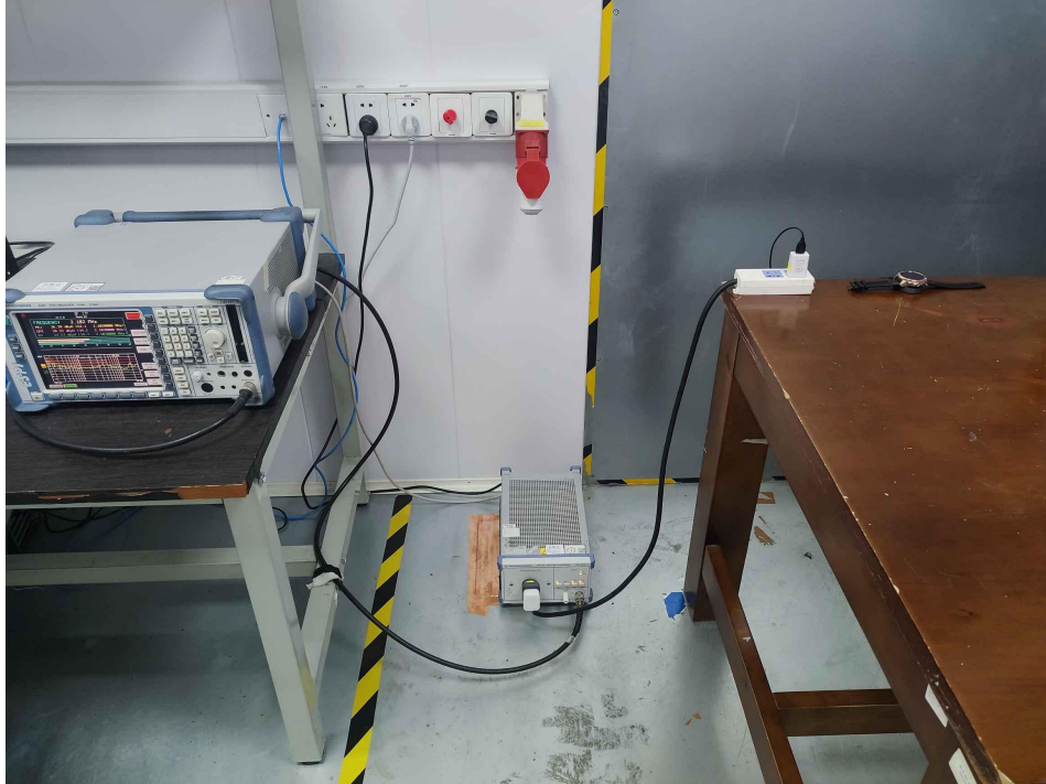
Conducted emissions at AC power line (150kHz-30MHz)
