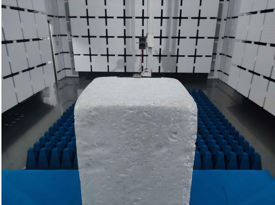
Radiated Emissions (above 1GHz)
