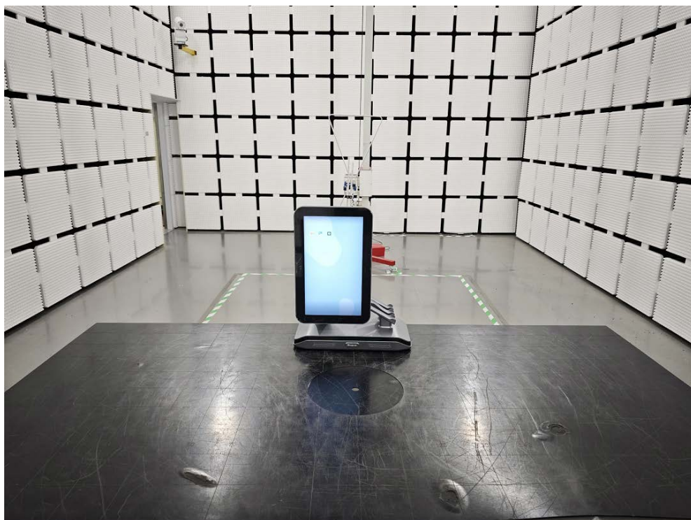
Spurious Radiation Emissions Test (<1G)
