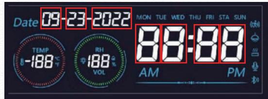
Long press (S) to enter the Settings mode, then short tap (S) to set the time, the digits on the screen flashing. Tap the (S) to change the digits, long tap it to switch to the next option
