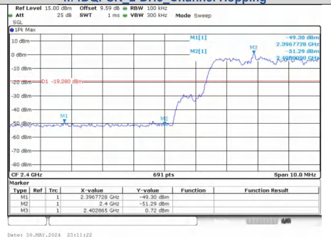
Out Of Band Emission(Left) \pi/4 DQPSK_2-DH5_Channel Hopping
