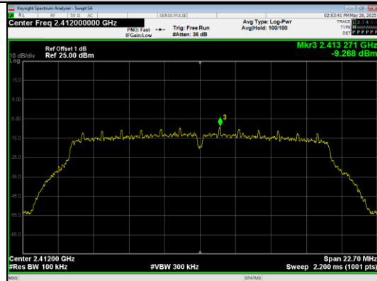
In-Band Reference Level IEEE 802.11g_Channel 1_20MHz_Antenna 0
