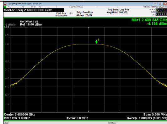
Peak Output Power BLE 1M_Channel 39
