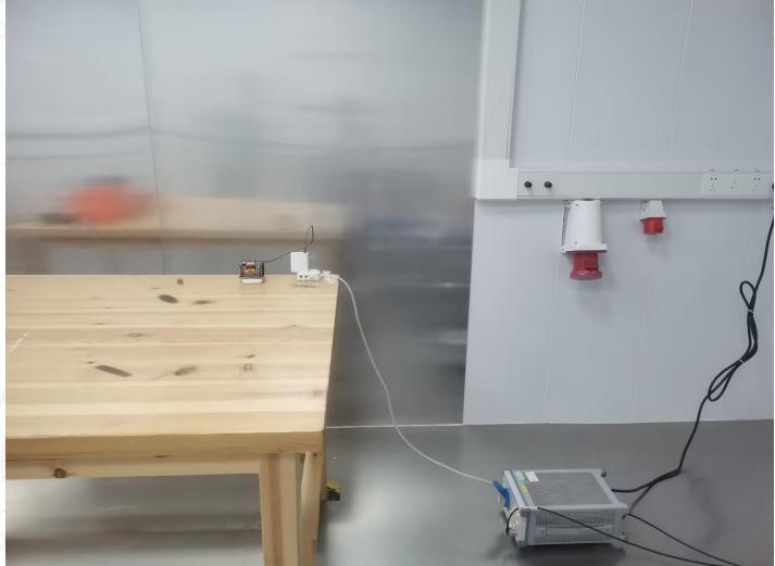
A photograph of a conducted emissions test setup. On the left, a wooden table holds a small electronic device connected to a power source. On the right, a power distribution unit with multiple outlets is connected to a large metal shielded enclosure. A power source is connected to the enclosure. A blue and white signal generator is on the floor to the right, connected to the setup. |
