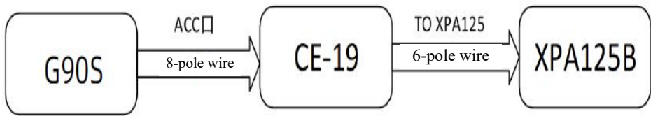
Schematic Diagram of Wiring between G90S and XPA125B
