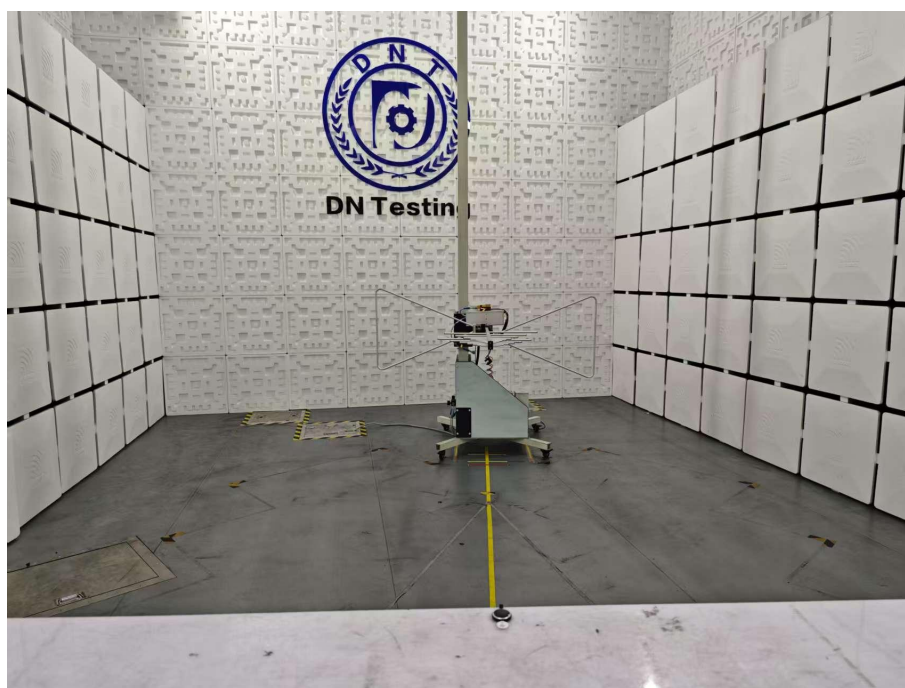
Radiated Emission Test View|(Below 1G)
