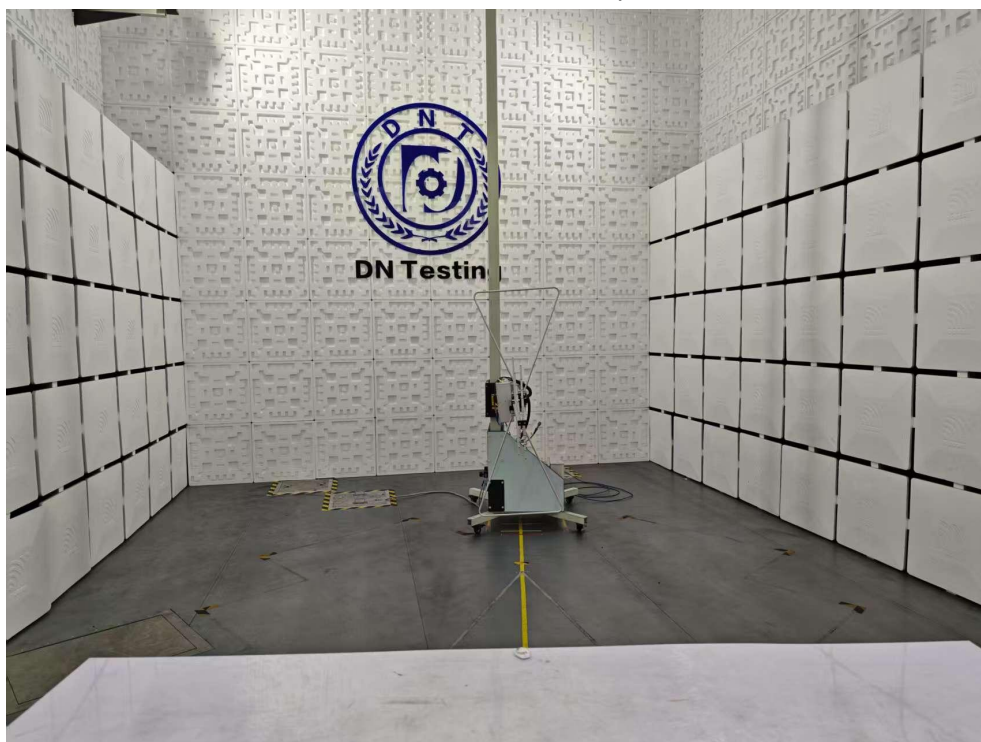
Radiated Emission Test View|(Below 1G)
