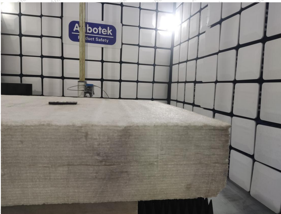
Photo of Radiation Emission Test (above 1GHz)
