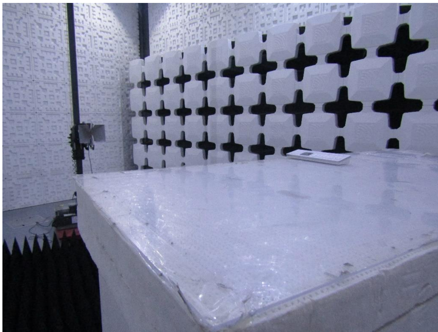
Radiated Emission (Above 1GHz)
