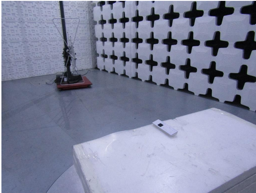
Radiated Emission (Above 1GHz)
