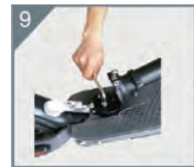
9. Tighten screw with a hexagonal wrench.
