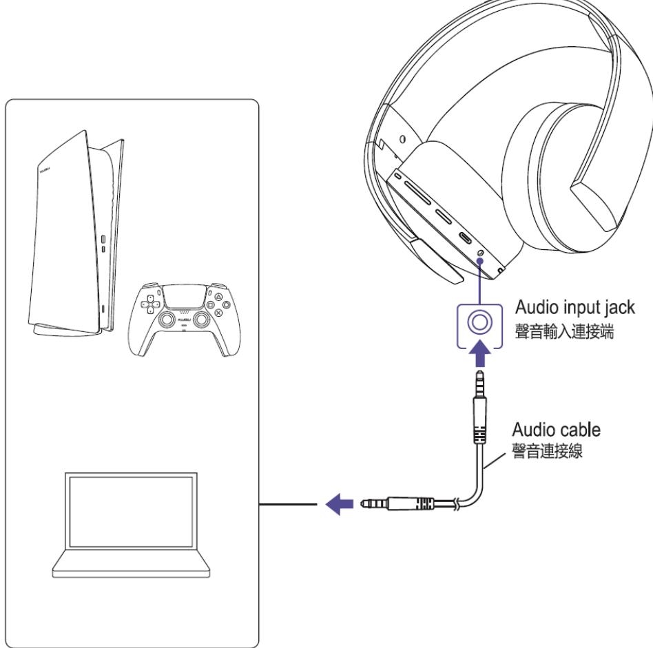
You can still use the headset to listen to game audio and chat with the microphones when you use the included audio cable. For example, if the headset battery runs out, you can continue gaming by plugging the headset into your wireless controller with the included audio cable. The included audio cable might not work with some devices. 使用隨附的聲音連接線時，您仍可以使用耳機組聆聽遊戲音訊並透過麥克風聊天。例如，當耳機組的電池沒電了，您可利用隨附的聲音連接線，將耳機組插入無線控制器以繼續游玩遊戲。隨附的聲音連接線可能無法用於某些裝置。
