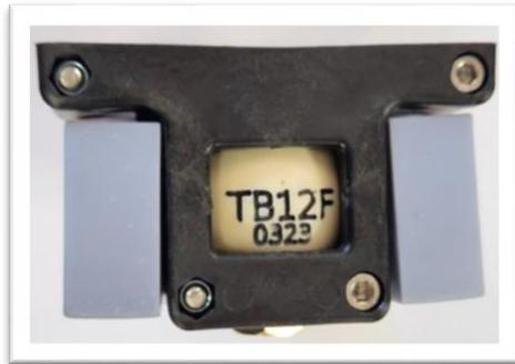
Place the sensor assembly in between the fork section of the mounting tool provided. As shown in images below.
