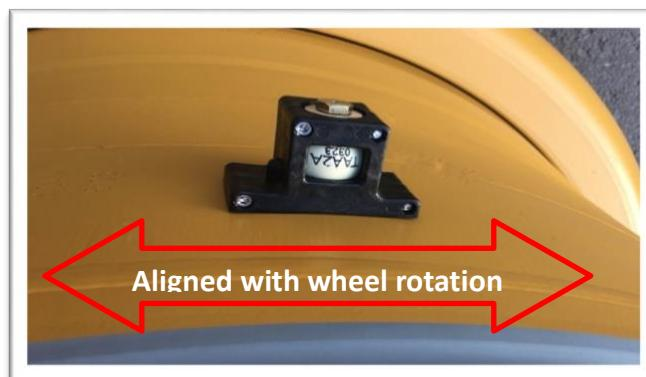
**NOTE: The sensor assembly must be orientated side on to the direction of wheel rotation as shown below.**
