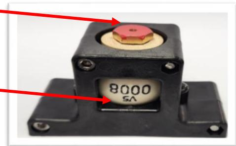
**Fitment:** The V5.0 sensor assembly is supplied preassembled and requires no further assembly or configuration. The Sensor will activate under pressurisation in the tyre.
