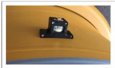
**Fitment Location:** Internal. Inside the wheel and tyre assembly. The sensor magnetically attaches to the rim base or bead seat band.
