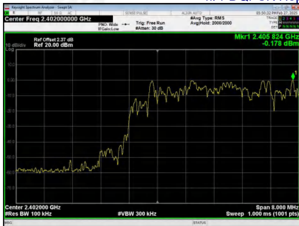
\pi/4 -DQPSK Hopping Band edge-left side
