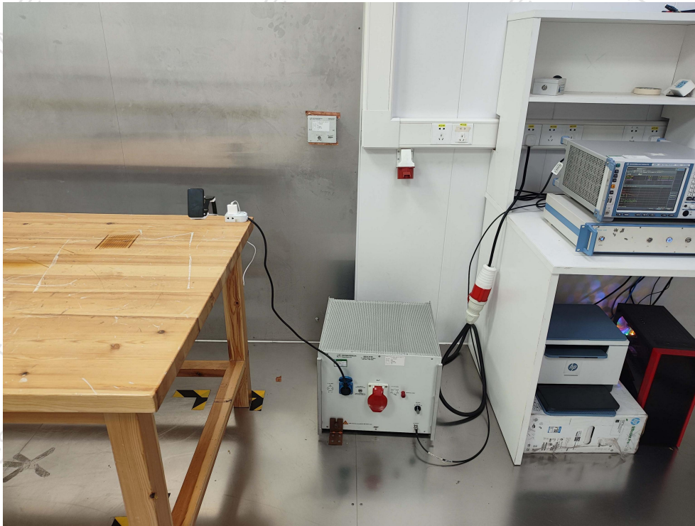
Photo of Conducted Emission Measurement
