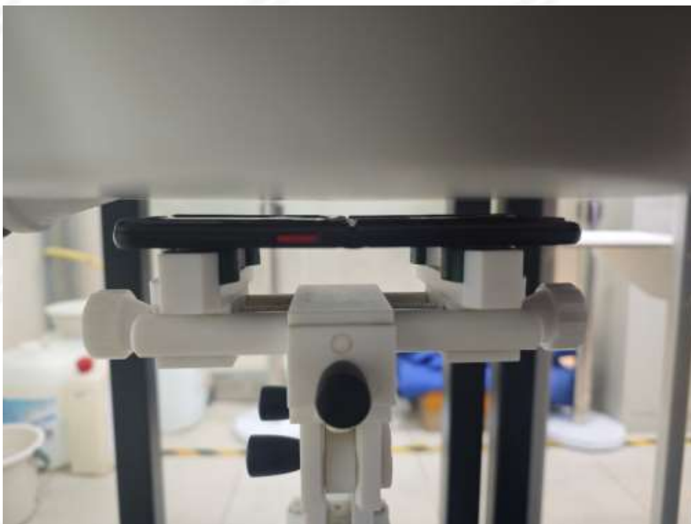
Body Back side(separation distance is 10mm)
