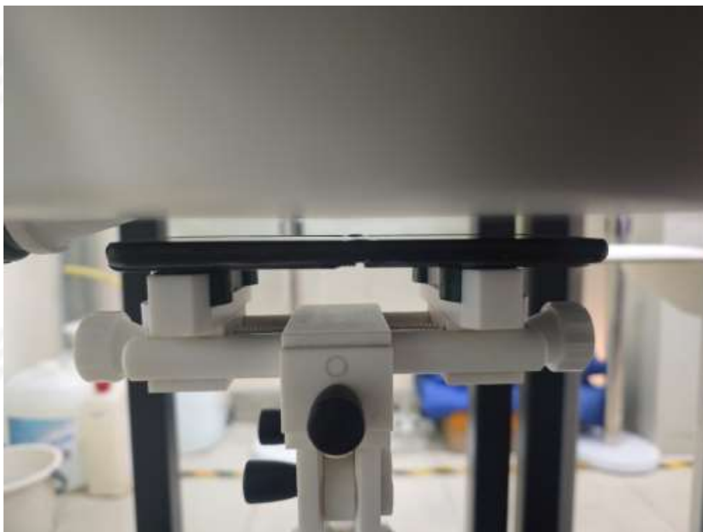
Body Front side(separation distance is 10mm)
