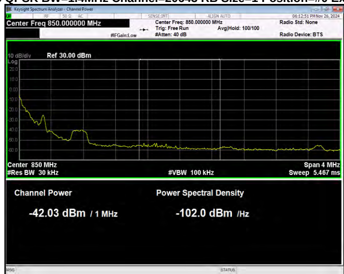
Band5 QPSK BW=1.4MHz Channel=20643 RB Size=1 Position=#0 Normal
