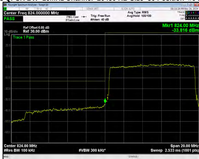
Band5 QPSK BW=10MHz Channel=20600 RB Size=50 Position=#0 Extended
