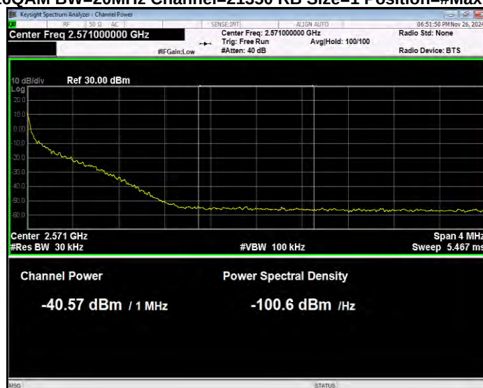
Band7 16QAM BW=5MHz Channel=20775 RB Size=1 Position=#0 Normal
