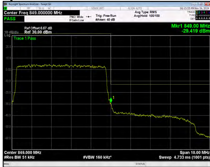
Band5 QPSK BW=5MHz Channel=20625 RB Size=25 Position=#0 Extended
