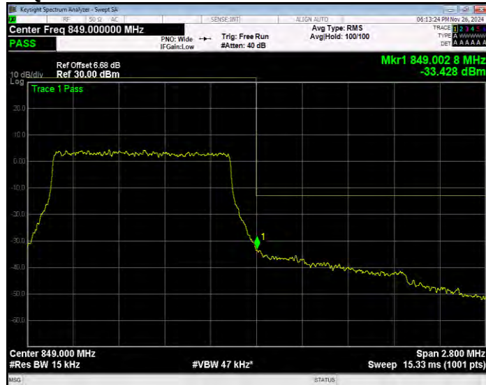
Band5 16QAM BW=1.4MHz Channel=20643 RB Size=1 Position=#Max Normal
