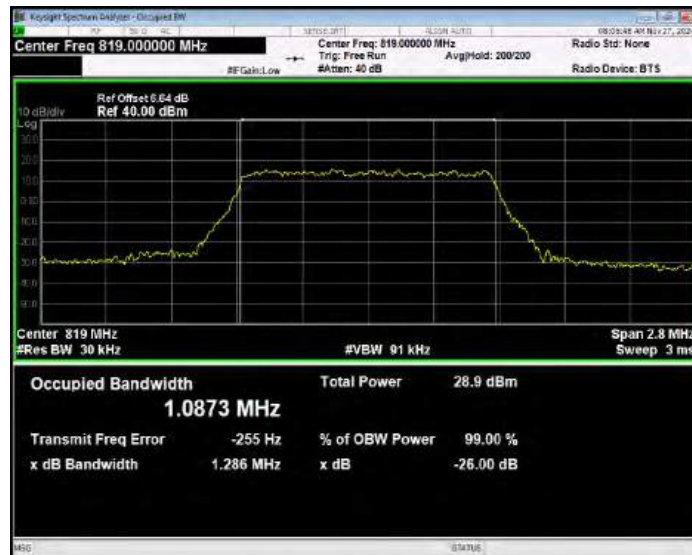
Band26(814-824) QPSK BW=1.4MHz Channel=26697 RB Size=6 Position=#0
