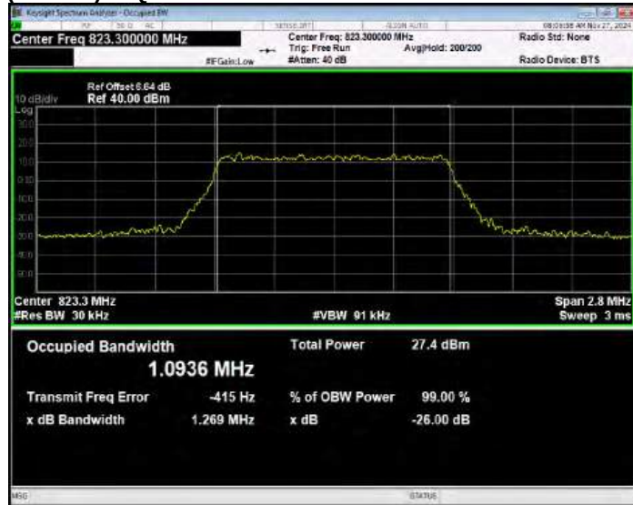
Band26(814-824) 16QAM BW=10MHz Channel=26740 RB Size=50 Position=#0
