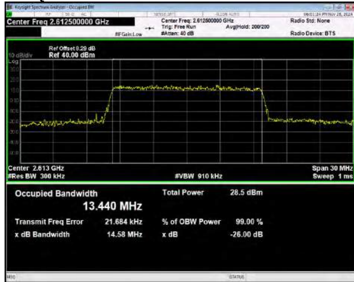
Band38 QPSK BW=15MHz Channel=38000 RB Size=75 Position=#0
