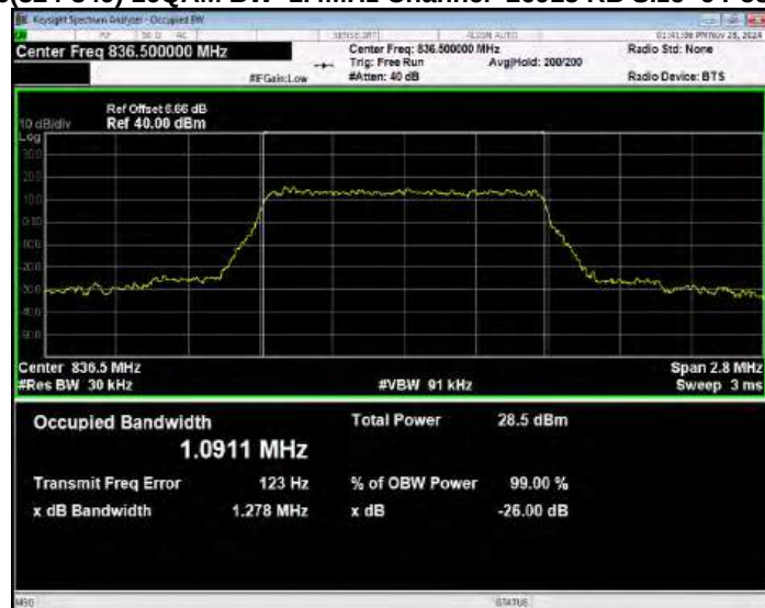
Band26(824-849) 16QAM BW=1.4MHz Channel=26797 RB Size=6 Position=#0
