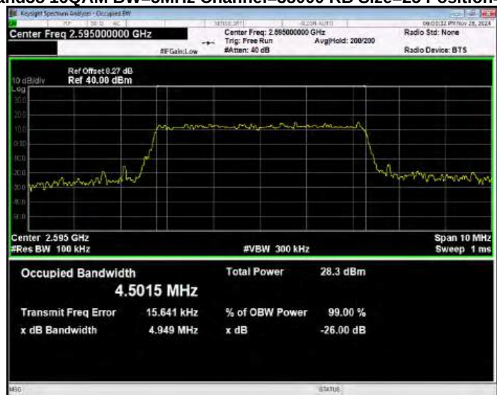
Band38 16QAM BW=5MHz Channel=38225 RB Size=25 Position=#0
