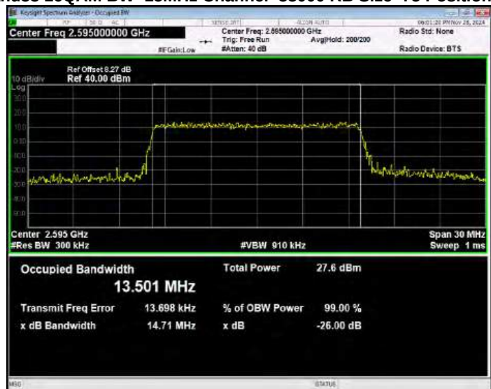
Band38 16QAM BW=15MHz Channel=38175 RB Size=75 Position=#0
