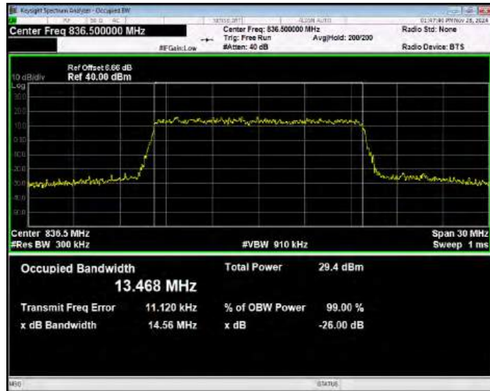
Band26(824-849) QPSK BW=15MHz Channel=26865 RB Size=75 Position=#0
