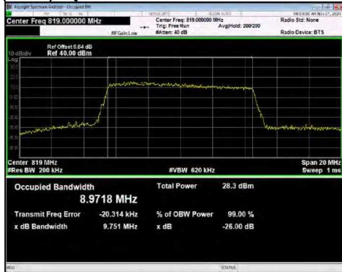
Band26(814-824) 16QAM BW=5MHz Channel=26740 RB Size=25 Position=#0
