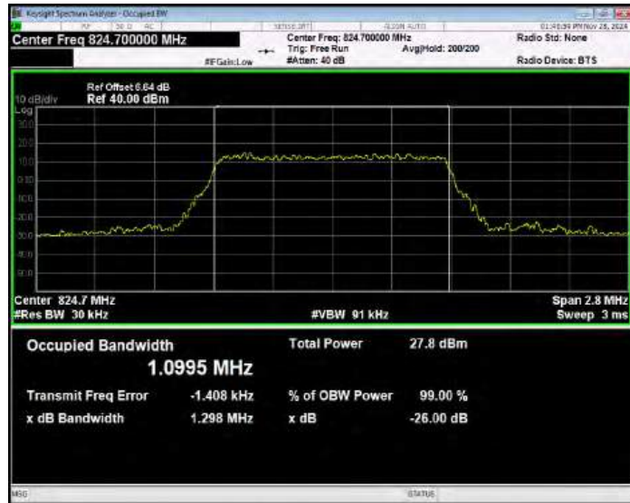
Band26(824-849) 16QAM BW=10MHz Channel=26915 RB Size=50 Position=#0
