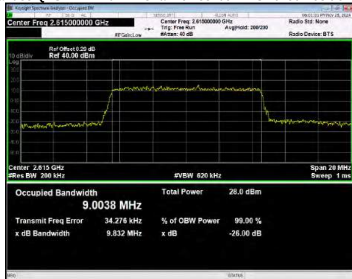
Band38 QPSK BW=15MHz Channel=37825 RB Size=75 Position=#0
