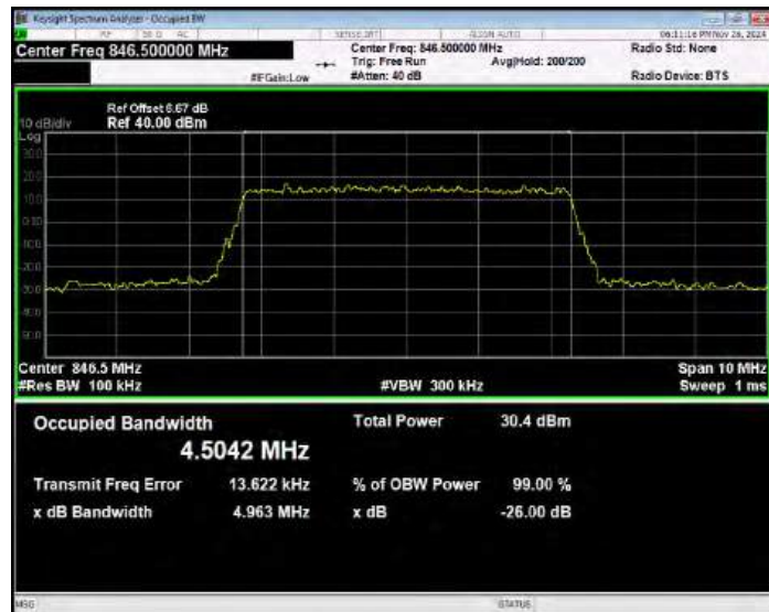
Band5 QPSK BW=5MHz Channel=20525 RB Size=25 Position=#0
