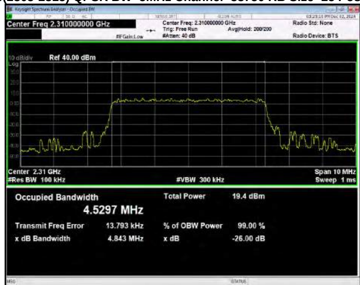
Band40(2305-2315) QPSK BW=5MHz Channel=38725 RB Size=25 Position=#0
