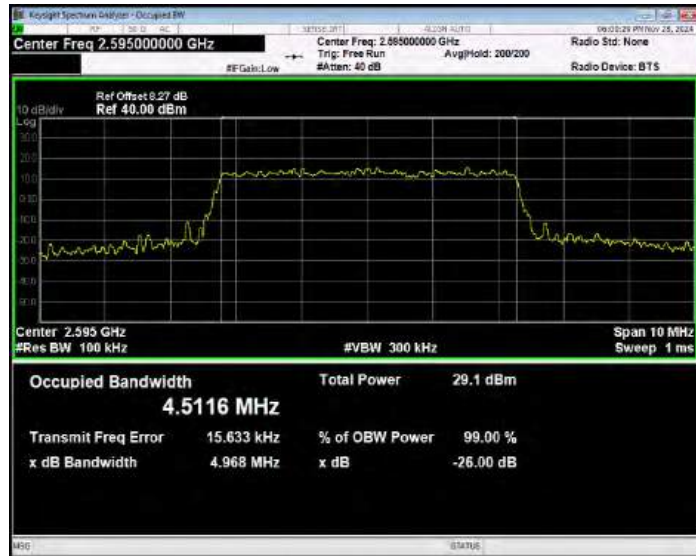
Band38 QPSK BW=5MHz Channel=38225 RB Size=25 Position=#0
