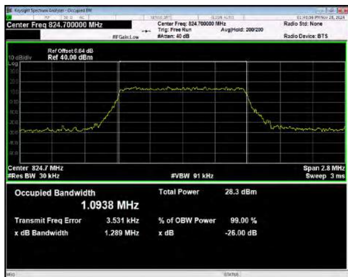
Band26(824-849) QPSK BW=1.4MHz Channel=26915 RB Size=6 Position=#0
