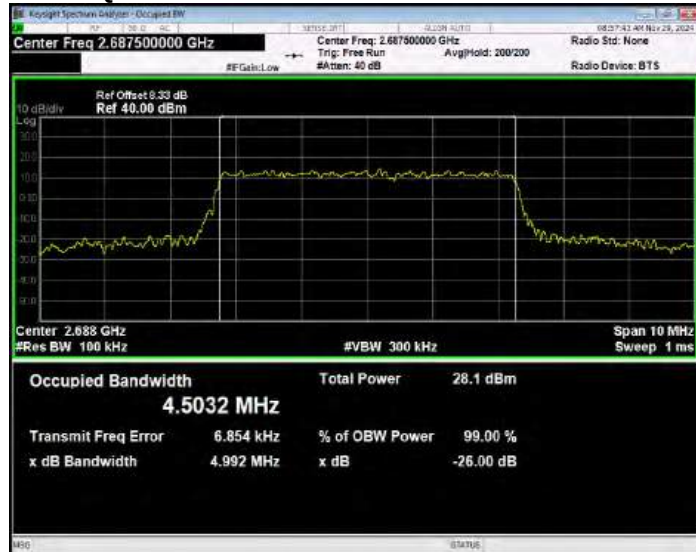
Band41 16QAM BW=5MHz Channel=40620 RB Size=25 Position=#0
