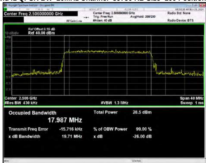
Band41 QPSK BW=5MHz Channel=41565 RB Size=25 Position=#0
