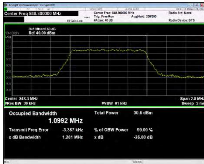
Band26(824-849) QPSK BW=10MHz Channel=26840 RB Size=50 Position=#0
