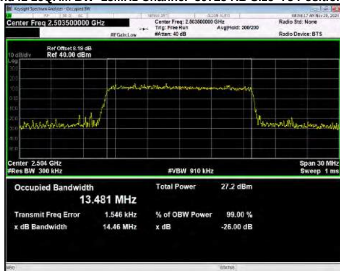
Band41 16QAM BW=20MHz Channel=41490 RB Size=100 Position=#0
