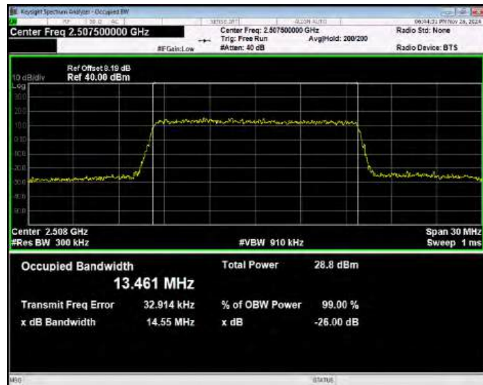
Band7 QPSK BW=10MHz Channel=21100 RB Size=50 Position=#0
