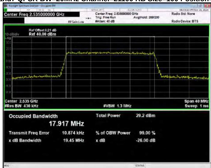
Band7 QPSK BW=20MHz Channel=20850 RB Size=100 Position=#0
