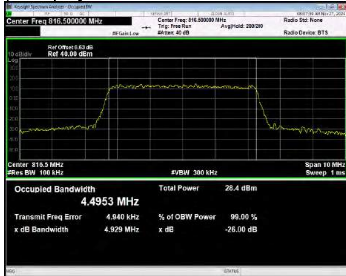
Band26(814-824) 16QAM BW=3MHz Channel=26775 RB Size=15 Position=#0
