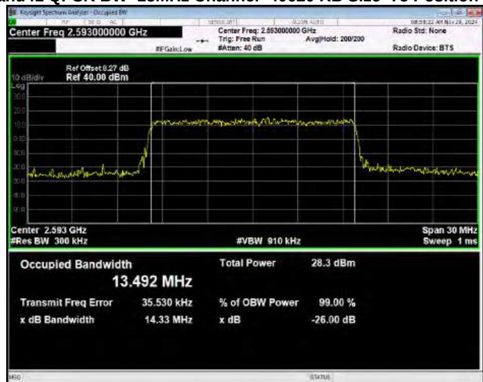
Band41 QPSK BW=15MHz Channel=39725 RB Size=75 Position=#0
