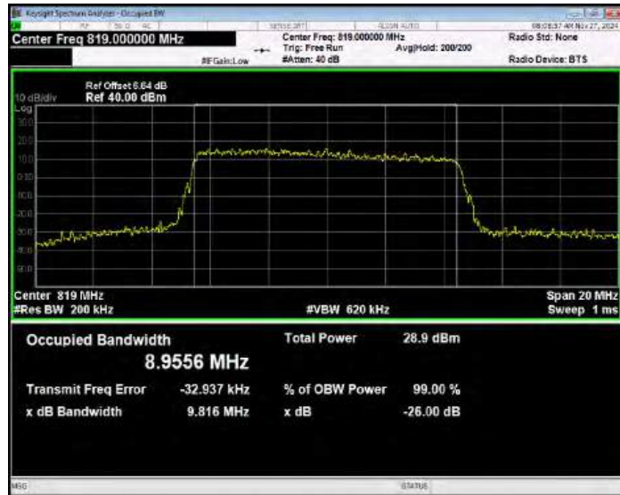
Band26(814-824) QPSK BW=5MHz Channel=26740 RB Size=25 Position=#0
