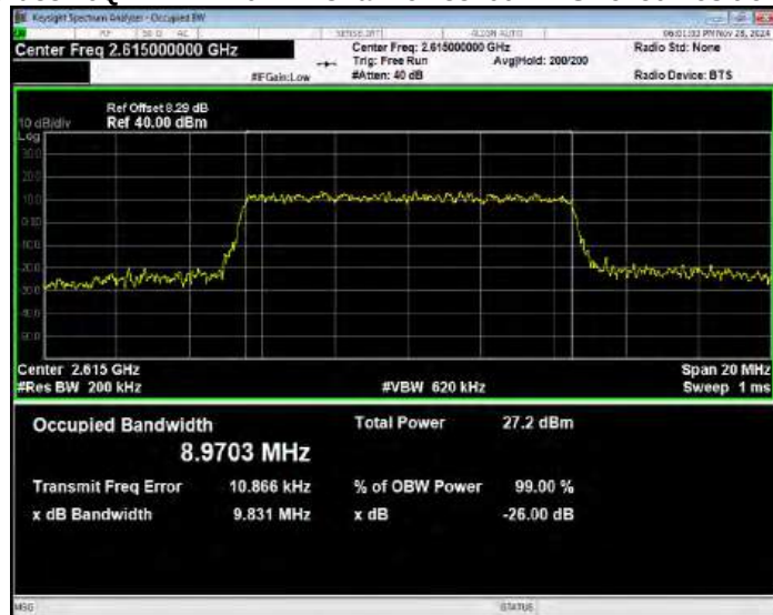
Band38 16QAM BW=15MHz Channel=37825 RB Size=75 Position=#0
