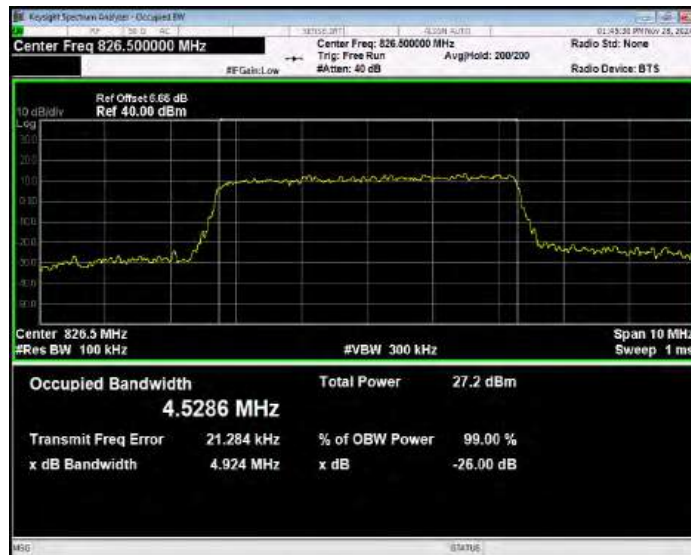
Band26(824-849) 16QAM BW=3MHz Channel=26805 RB Size=15 Position=#0
