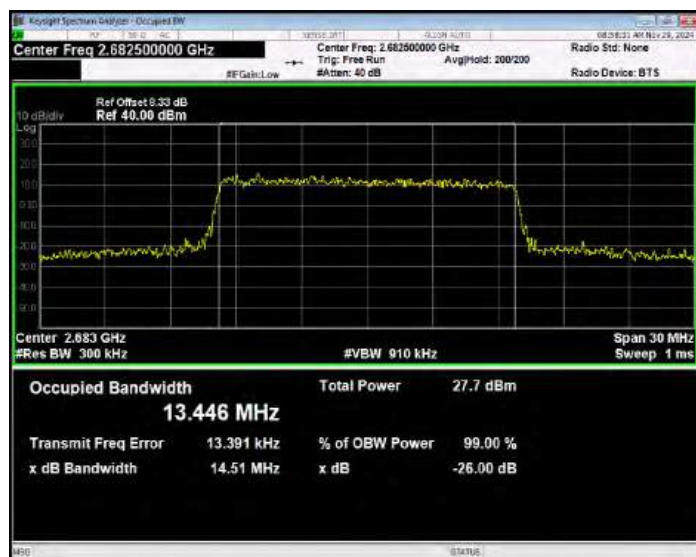
Band41 16QAM BW=10MHz Channel=41540 RB Size=50 Position=#0
