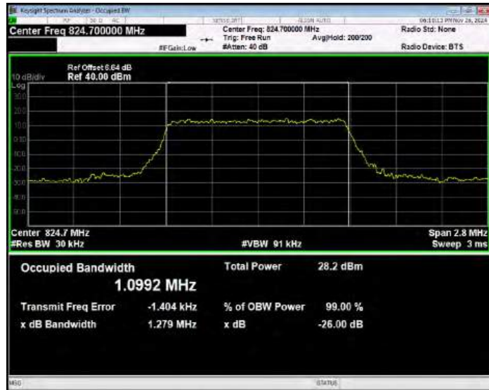
Band5 QPSK BW=1.4MHz Channel=20525 RB Size=6 Position=#0
