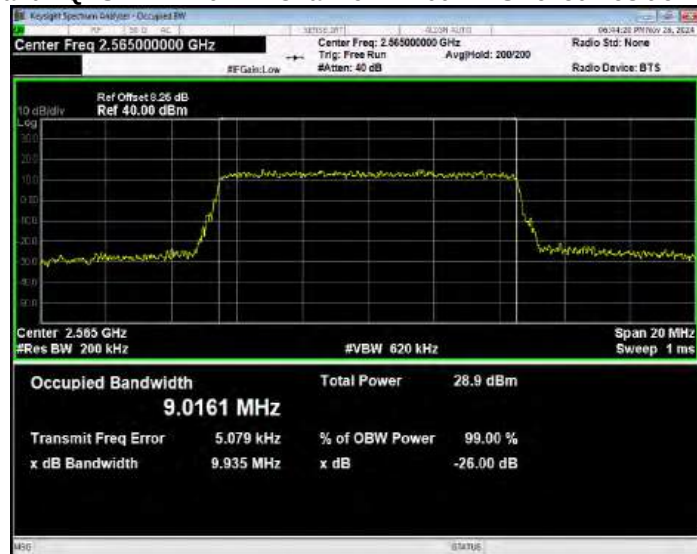
Band7 QPSK BW=20MHz Channel=21350 RB Size=100 Position=#0
