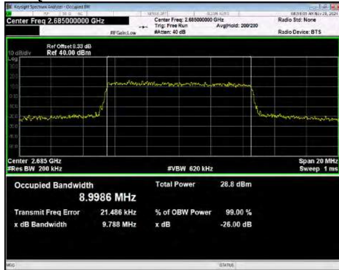
Band41 QPSK BW=20MHz Channel=40620 RB Size=100 Position=#0
