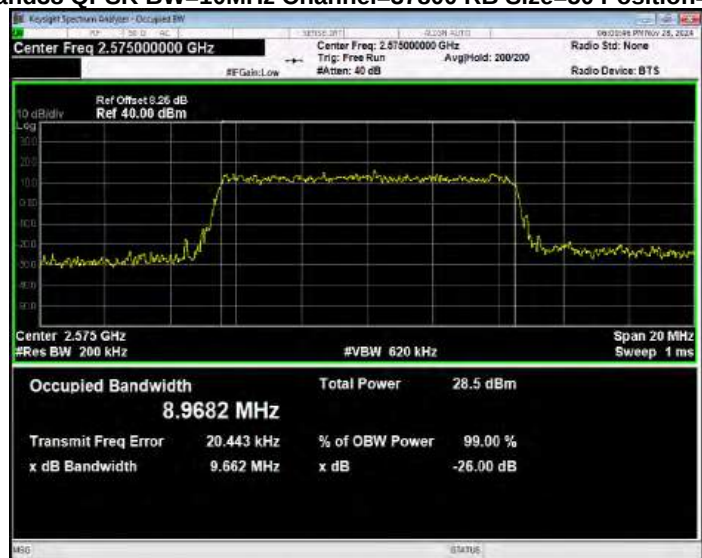
Band38 QPSK BW=10MHz Channel=38000 RB Size=50 Position=#0
