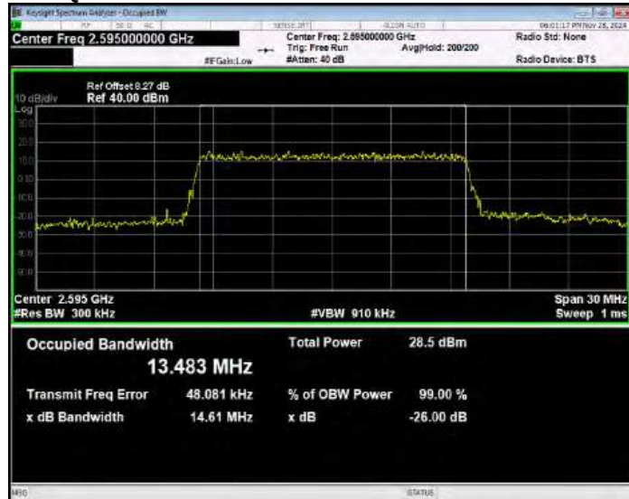
Band38 QPSK BW=5MHz Channel=38000 RB Size=25 Position=#0
