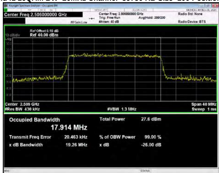
Band41 16QAM BW=20MHz Channel=40620 RB Size=100 Position=#0
