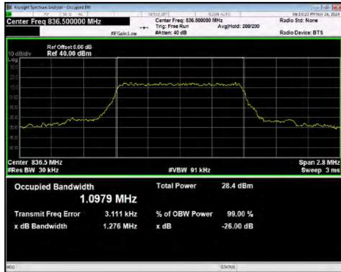
Band5 16QAM BW=1.4MHz Channel=20643 RB Size=6 Position=#0
