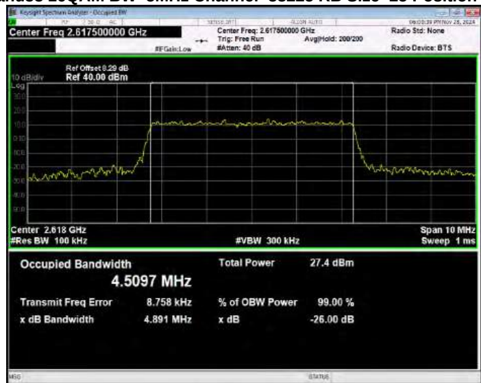
Band38 16QAM BW=20MHz Channel=38150 RB Size=100 Position=#0
