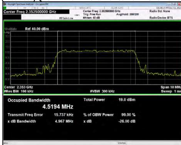
Band40(2350-2360) QPSK BW=10MHz Channel=39200 RB Size=50 Position=#0
