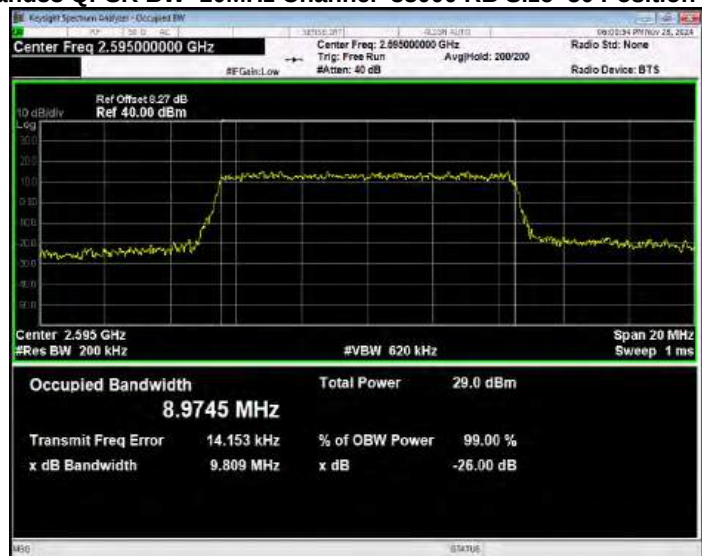
Band38 QPSK BW=20MHz Channel=37850 RB Size=100 Position=#0
