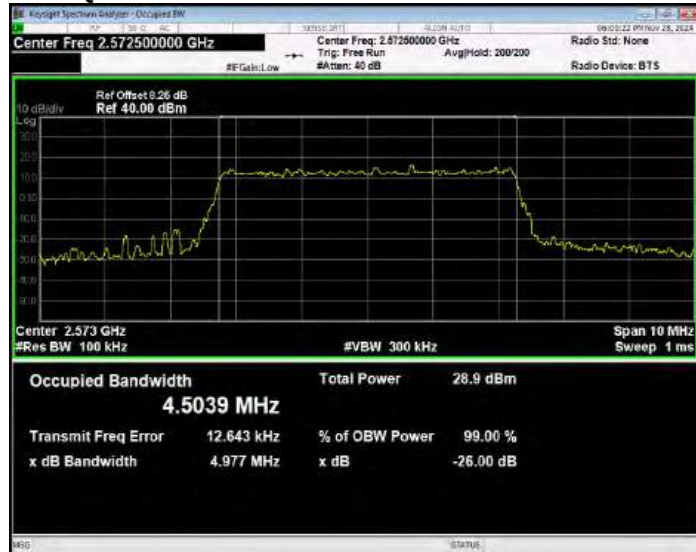
Band38 QPSK BW=20MHz Channel=38000 RB Size=100 Position=#0
