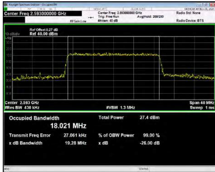
Band41 QPSK BW=10MHz Channel=39700 RB Size=50 Position=#0
