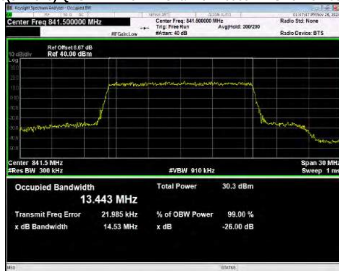
Band26(824-849) QPSK BW=15MHz Channel=26915 RB Size=75 Position=#0
