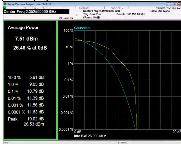
Band40(2350-2360) 16QAM BW=5MHz Channel=39200 RB Size=1 Position=#0
