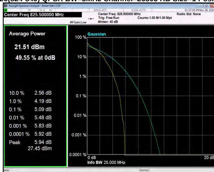
Band26(824-849) QPSK BW=3MHz Channel=26915 RB Size=1 Position=#0
