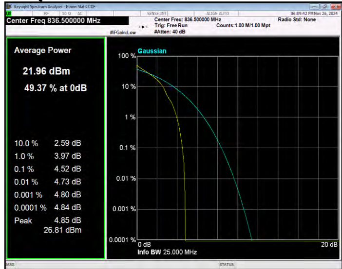
Band5 QPSK BW=10MHz Channel=20600 RB Size=1 Position=#0
