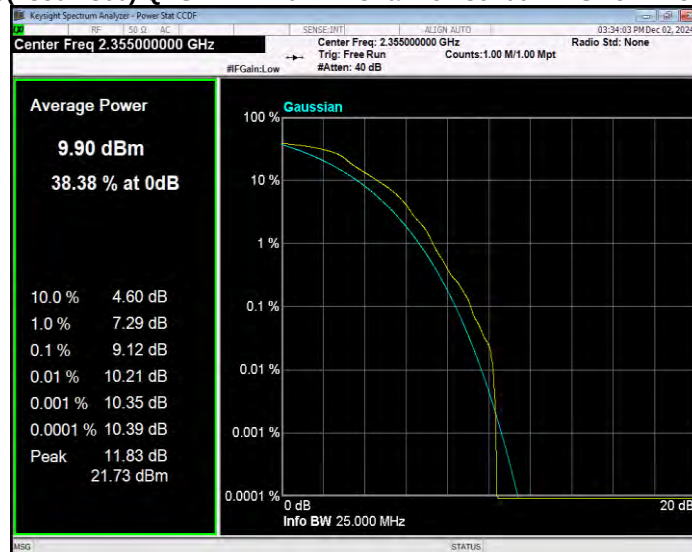
Band40(2350-2360) QPSK BW=5MHz Channel=39175 RB Size=1 Position=#0
