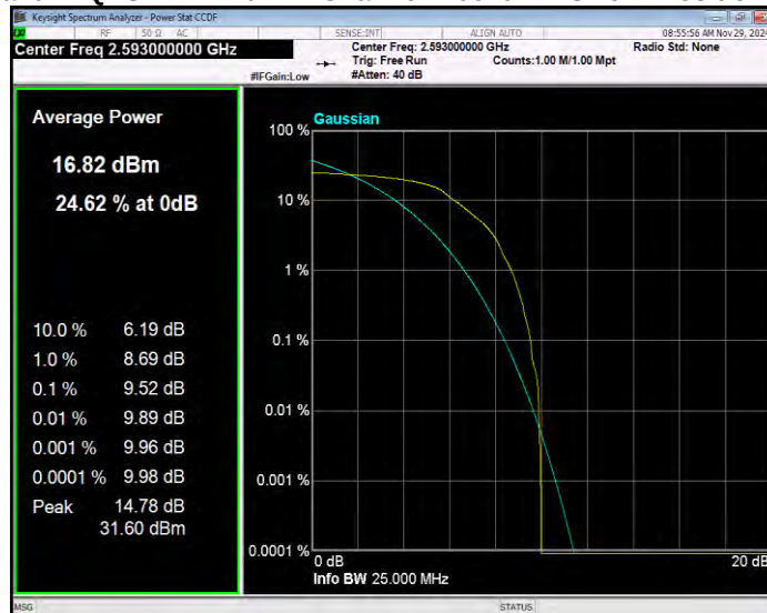
Band41 16QAM BW=5MHz Channel=40620 RB Size=1 Position=#0
