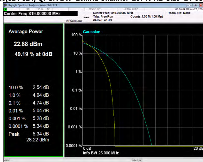
Band26(814-824) QPSK BW=1.4MHz Channel=26783 RB Size=1 Position=#0
