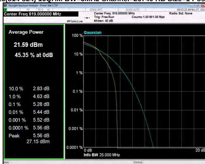
Band26(814-824) QPSK BW=10MHz Channel=26740 RB Size=1 Position=#0
