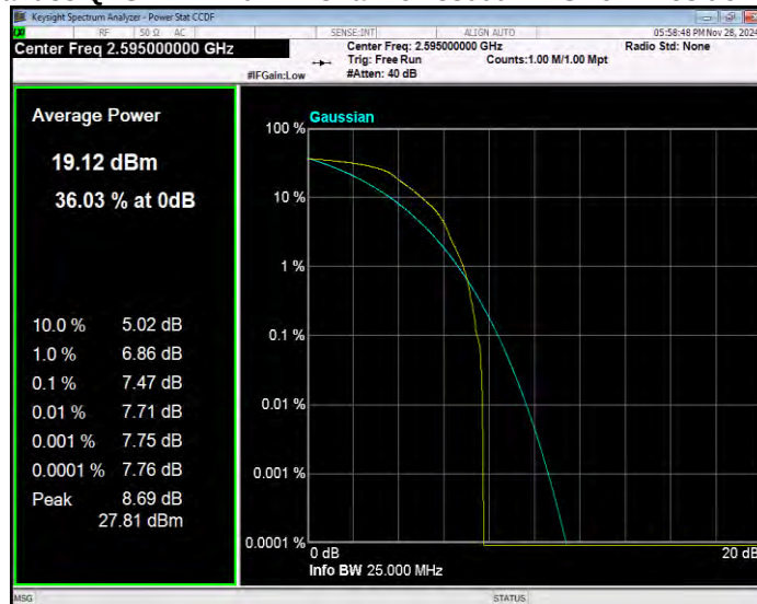
Band38 QPSK BW=10MHz Channel=38200 RB Size=1 Position=#0
