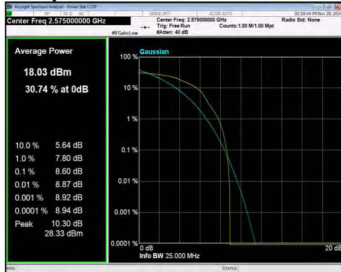
Band38 16QAM BW=15MHz Channel=37825 RB Size=1 Position=#0
