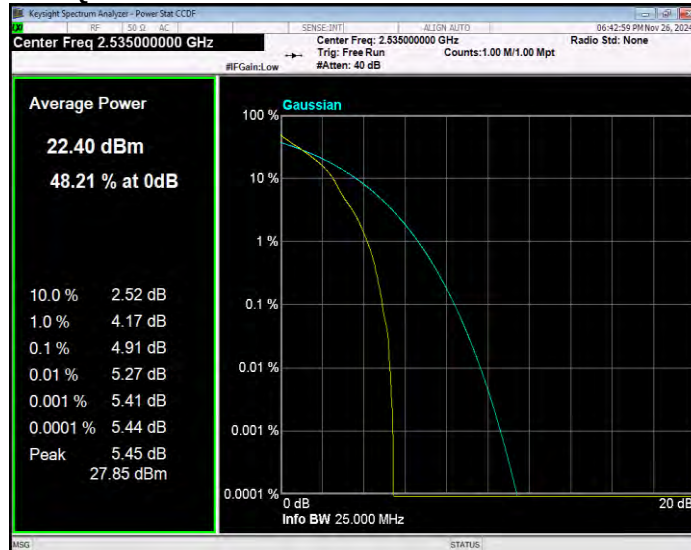
Band7 QPSK BW=15MHz Channel=21375 RB Size=1 Position=#0
