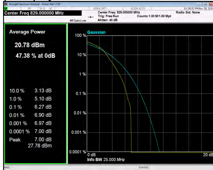
Band26(824-849) 16QAM BW=10MHz Channel=26915 RB Size=1 Position=#0
