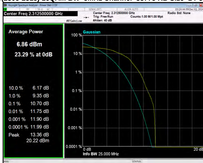
Band40(2305-2315) 16QAM BW=5MHz Channel=38750 RB Size=1 Position=#0
