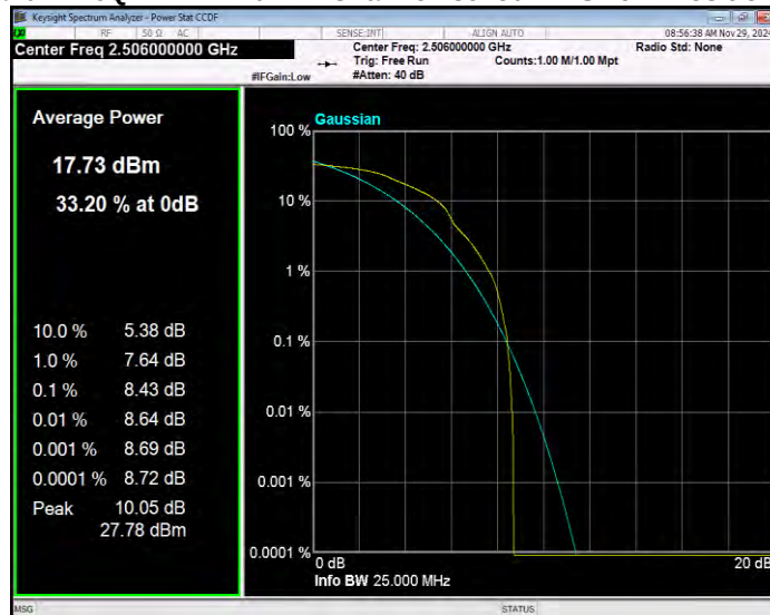
Band41 16QAM BW=20MHz Channel=40620 RB Size=1 Position=#0
