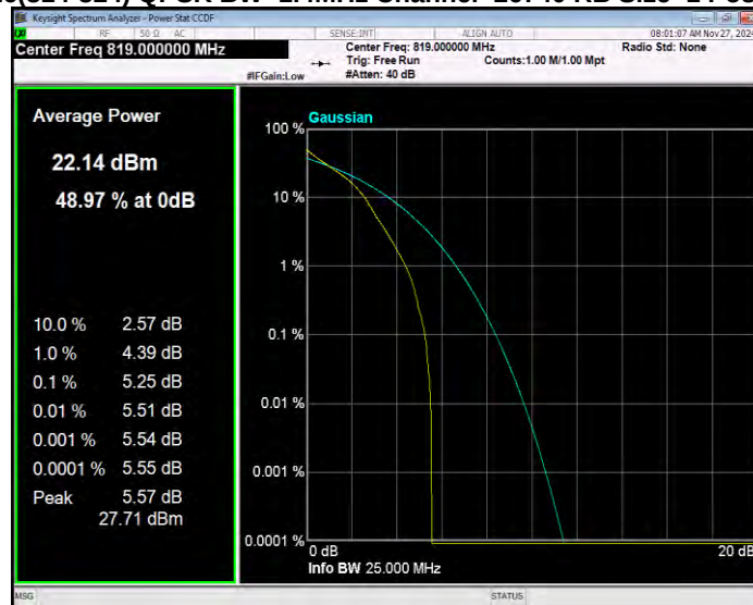
Band26(814-824) QPSK BW=5MHz Channel=26715 RB Size=1 Position=#0
