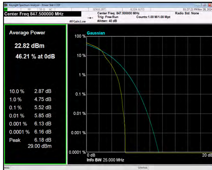
Band26(824-849) QPSK BW=1.4MHz Channel=26797 RB Size=1 Position=#0
