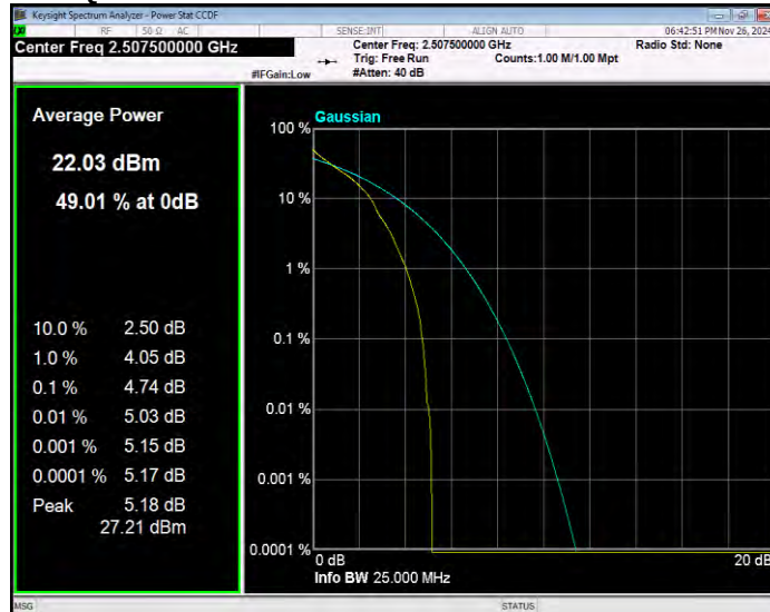
Band7 QPSK BW=10MHz Channel=21400 RB Size=1 Position=#0
