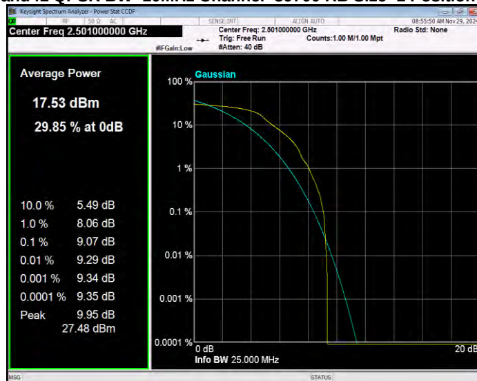
Band41 QPSK BW=10MHz Channel=40620 RB Size=1 Position=#0
