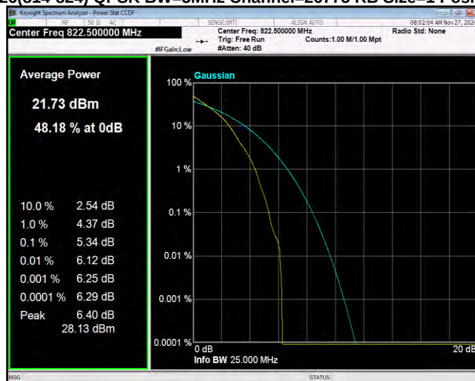
Band26(814-824) QPSK BW=3MHz Channel=26705 RB Size=1 Position=#0
