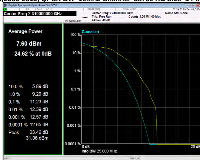
Band40(2305-2315) 16QAM BW=5MHz Channel=38775 RB Size=1 Position=#0
