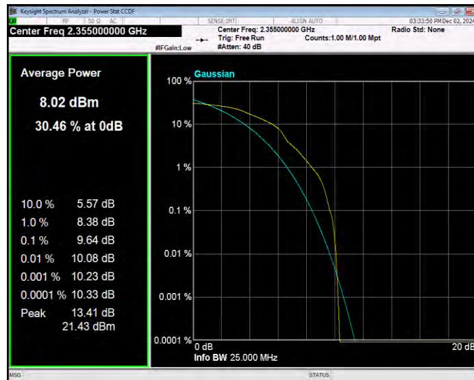
Band40(2350-2360) QPSK BW=5MHz Channel=39225 RB Size=1 Position=#0
