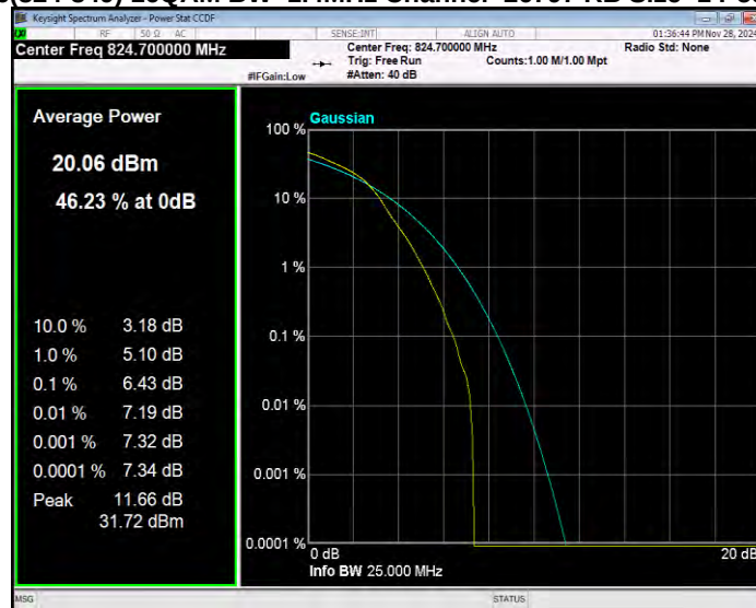
Band26(824-849) 16QAM BW=10MHz Channel=26990 RB Size=1 Position=#0
