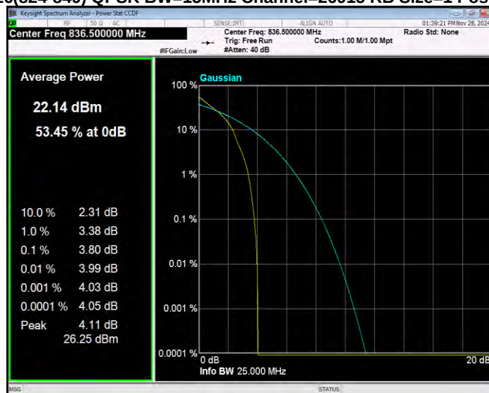
Band26(824-849) QPSK BW=15MHz Channel=26965 RB Size=1 Position=#0
