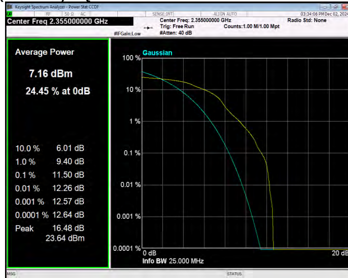
Band40(2350-2360) QPSK BW=10MHz Channel=39200 RB Size=1 Position=#0
