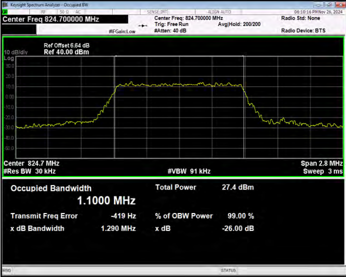
Band5 16QAM BW=10MHz Channel=20450 RB Size=50 Position=#0
