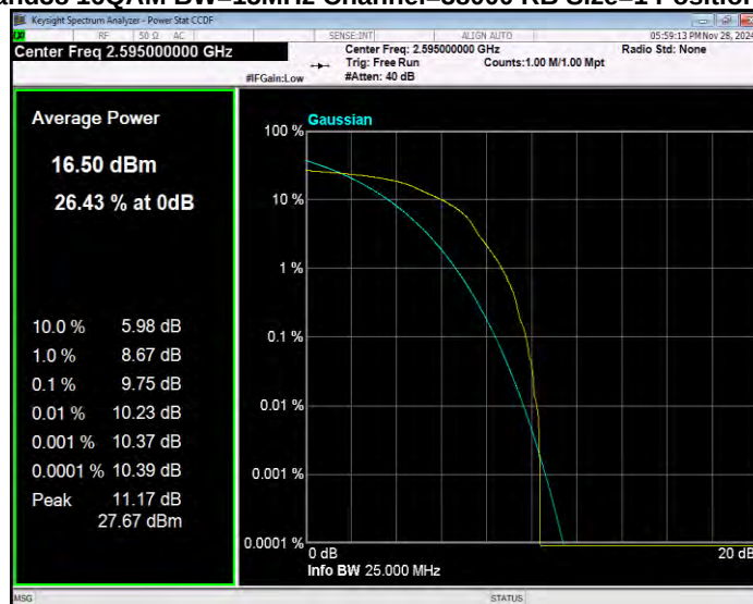
Band38 16QAM BW=10MHz Channel=38000 RB Size=1 Position=#0
