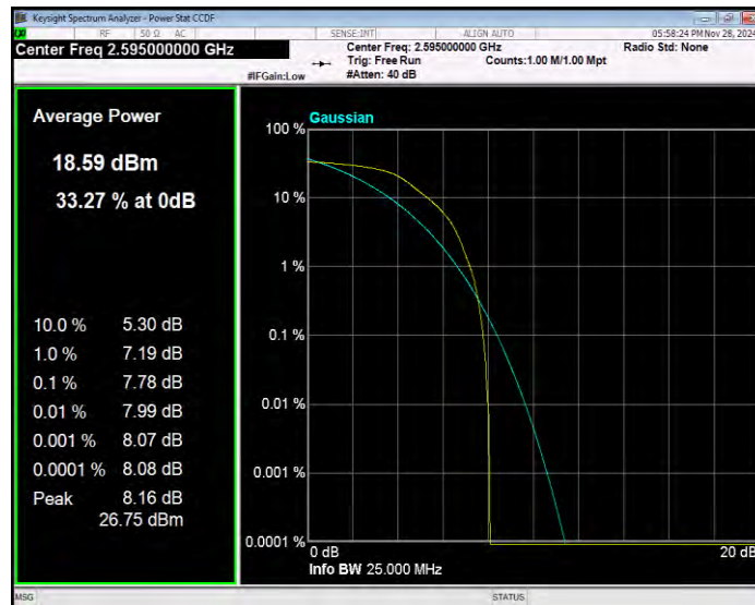
Band38 QPSK BW=5MHz Channel=37775 RB Size=1 Position=#0
