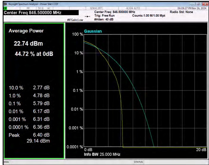
Band5 QPSK BW=10MHz Channel=20525 RB Size=1 Position=#0
