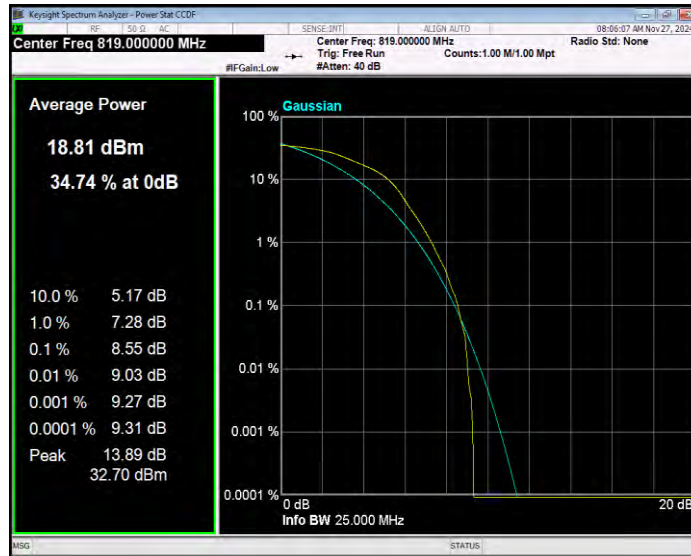
Band26(814-824) 16QAM BW=3MHz Channel=26775 RB Size=1 Position=#0
