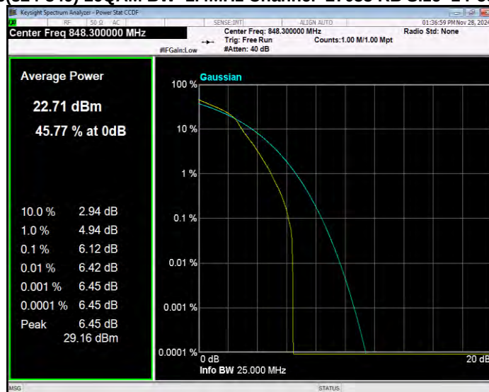
Band26(824-849) 16QAM BW=1.4MHz Channel=26915 RB Size=1 Position=#0
