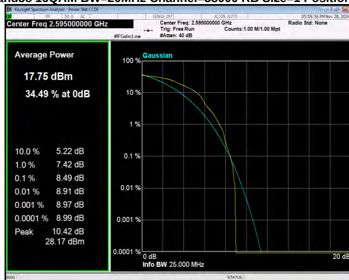
Band38 16QAM BW=20MHz Channel=38150 RB Size=1 Position=#0
