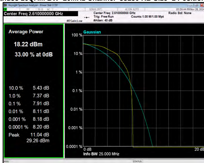
Band38 16QAM BW=15MHz Channel=38175 RB Size=1 Position=#0
