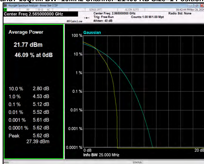
Band7 16QAM BW=20MHz Channel=21100 RB Size=1 Position=#0
