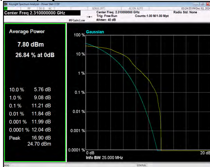
Band40(2305-2315) 16QAM BW=5MHz Channel=38725 RB Size=1 Position=#0
