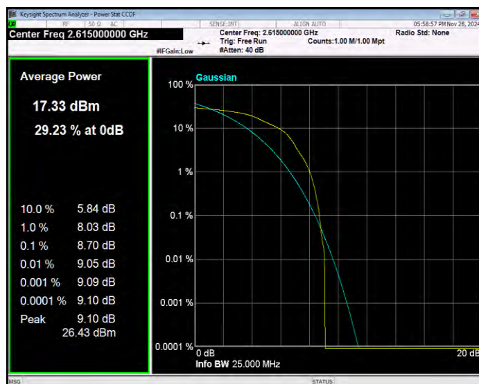
Band38 16QAM BW=20MHz Channel=38000 RB Size=1 Position=#0
