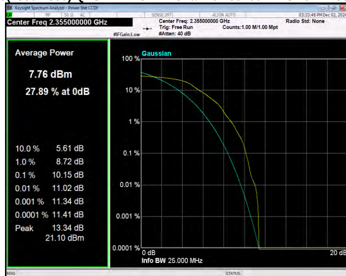
Band41 16QAM BW=10MHz Channel=40620 RB Size=1 Position=#0
