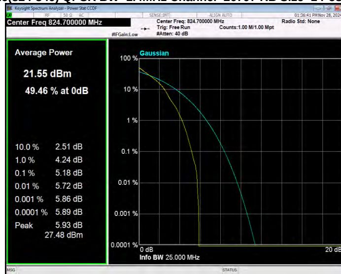
Band26(824-849) 16QAM BW=5MHz Channel=27015 RB Size=1 Position=#0
