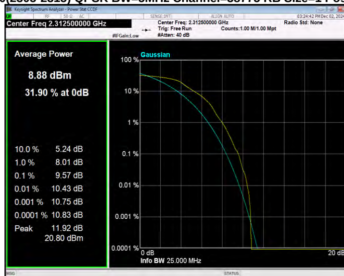
Band40(2305-2315) QPSK BW=5MHz Channel=38750 RB Size=1 Position=#0
