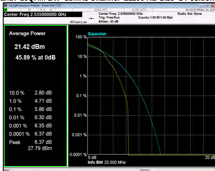
Band7 16QAM BW=15MHz Channel=20825 RB Size=1 Position=#0
