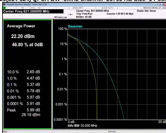
Band26(824-849) 16QAM BW=1.4MHz Channel=27033 RB Size=1 Position=#0
