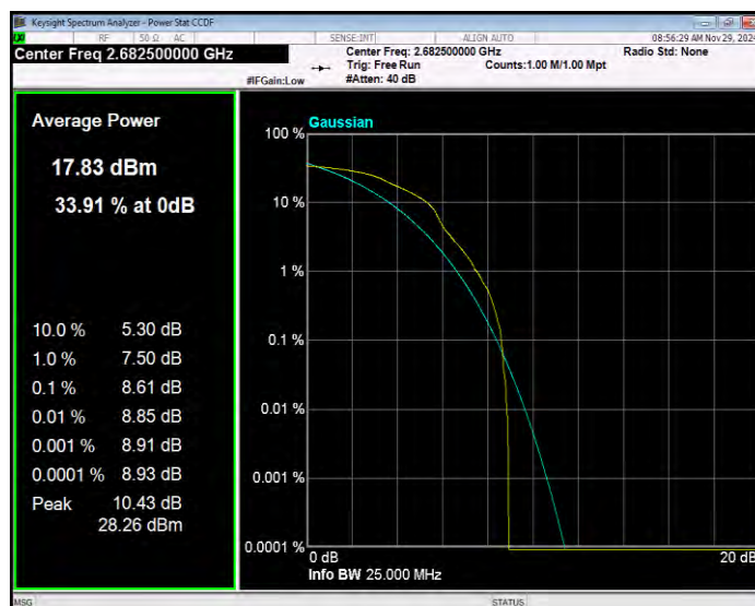
Band41 16QAM BW=10MHz Channel=41540 RB Size=1 Position=#0
