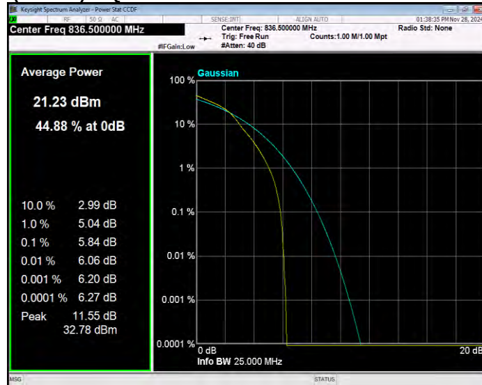
Band26(824-849) 16QAM BW=5MHz Channel=26815 RB Size=1 Position=#0
