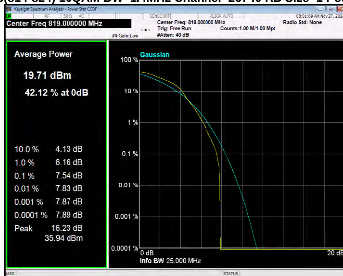
Band26(814-824) 16QAM BW=1.4MHz Channel=26697 RB Size=1 Position=#0
