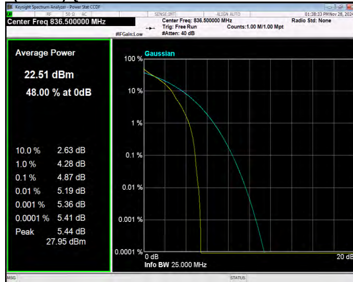
Band38 16QAM BW=10MHz Channel=37800 RB Size=1 Position=#0
