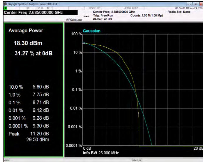
Band41 16QAM BW=15MHz Channel=39725 RB Size=1 Position=#0
