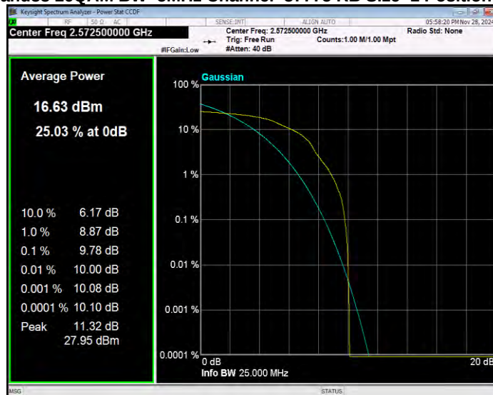
Band38 16QAM BW=5MHz Channel=38000 RB Size=1 Position=#0
