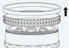
2. Remove the middle threaded ring in the direction of the arrow.
