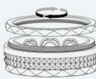
3. Rotate in the direction of the arrow to assemble the top threaded ring.
