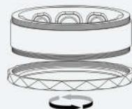
1. Rotate in the direction of the arrow to assemble the bottom threaded ring.
