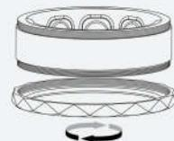
3. Rotate in the direction of the arrow to remove the bottom threaded ring.
