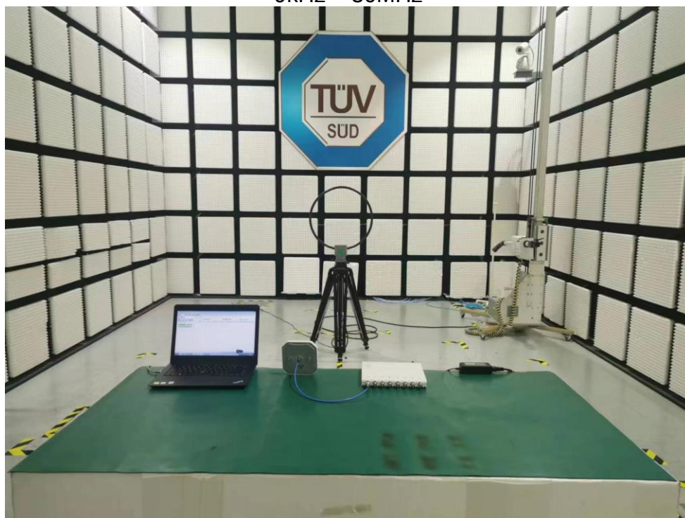
Radiated Emission Setup 9kHz ~ 30MHz
