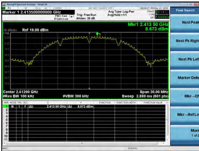
802.11b LOW CHANNEL, CARRIER LEVEL
