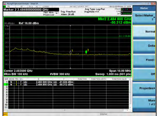
802.11b HIGH CHANNEL, BAND EDGE
