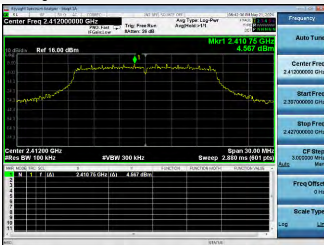
802.11g LOW CHANNEL, CARRIER LEVEL
