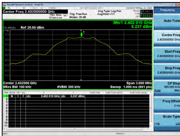
GFSK (BLE 1Mbps) LOW CHANNEL, CARRIER LEVEL
