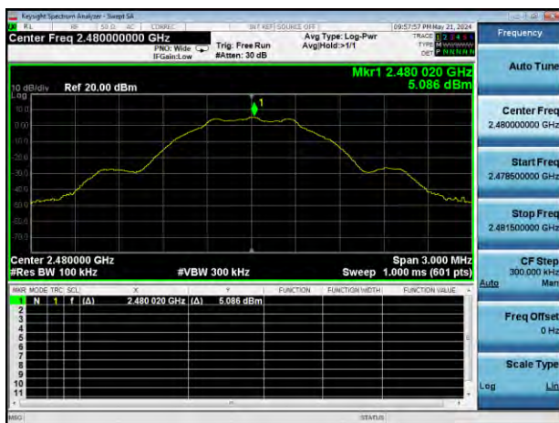
GFSK (BLE 1Mbps) HIGH CHANNEL, CARRIER LEVEL
