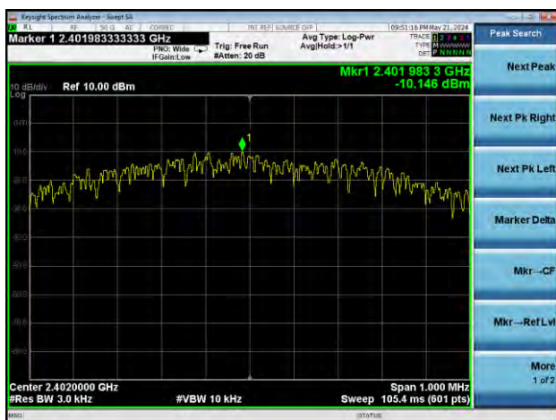
GFSK (BLE 1Mbps) LOW CHANNEL
