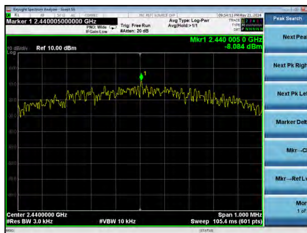
GFSK (BLE 1Mbps) MIDDLE CHANNEL
