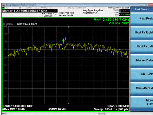
GFSK (BLE 1Mbps) HIGH CHANNEL
