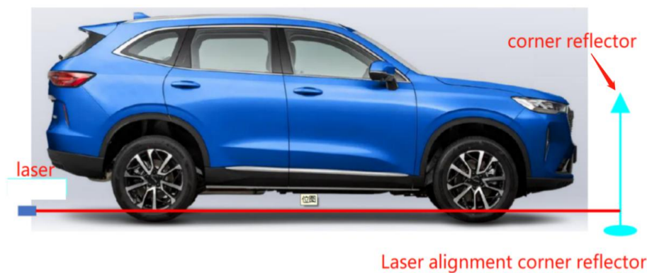
Figure 12. Ensure that the corner reflector support rod is at the laser irradiation point
