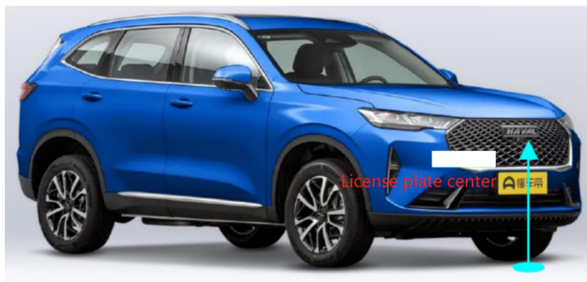
Figure 9.Place the corner reflector in the center of the front of the vehicle
