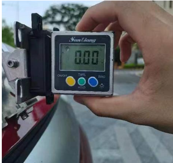
Figure 6. Pitch angle adjustment not exceeding \pm 2^\circ
