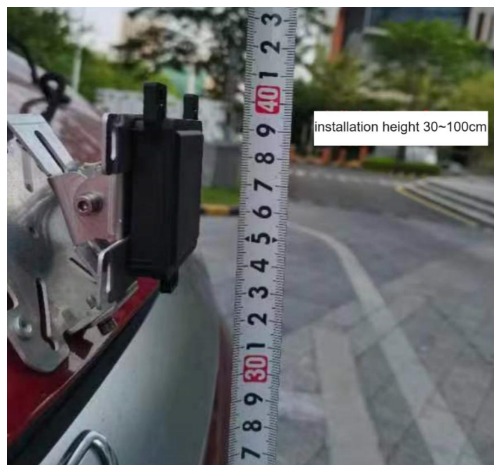
Figure 3. Radar installation height selection 30cm---100cm
