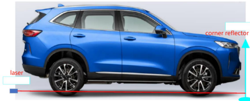
Figure 10. Find the centerline of the vehicle body
