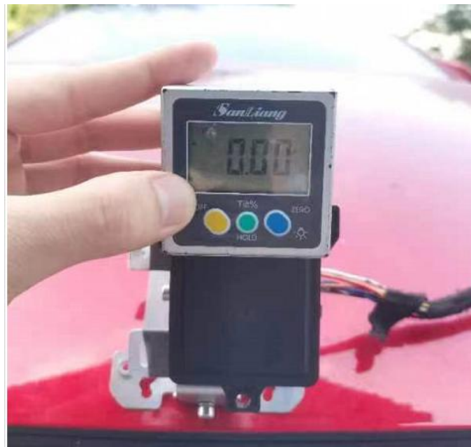
Figure 5. Horizontal angle adjustment not exceeding \pm 2^\circ
