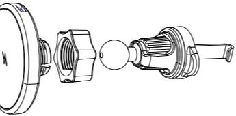
3. The assembled magnetic car wireless charging bracket, installed in the car air conditioning vent position to connect the USB cable, this time the indicator state for the blue light is on for 60 seconds after the off.
