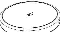
4. After powering up, when the phone is placed on it, it enters the wireless charging state. At this time the indicator light for the blue light breathing 60 seconds after the off.
