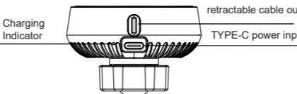
3. The assembled magnetic car wireless charging bracket, installed in the car in the air conditioning vent position connected to the USB cable, this time the status of the indicator for the blue light is on for 5 seconds after the light goes out.
