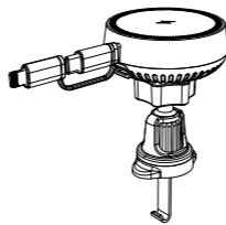
4. When the phone is put on, it enters the wireless charging state. At this time the indicator light is blue light always on.
