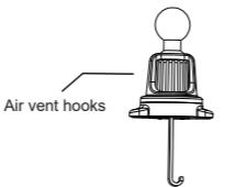
2. After taking out the air outlet hook, align the mounting nut position and turn the nut to tighten the air outlet hook.
