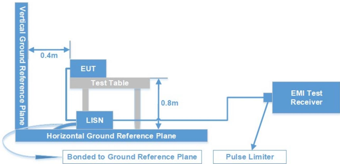
The setup of EUT is according with per ANSI C63.10-2013 measurement procedure. The specification used was with the FCC Part 15.207 limits.
