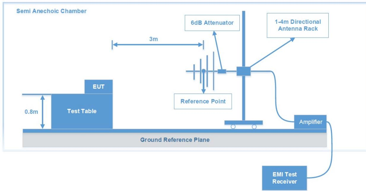
The radiated emission tests were performed in the 3-meter chamber a test site, using the setup accordance with the ANSI C63.10. The specification used was the FCC Part Subpart C limits.
