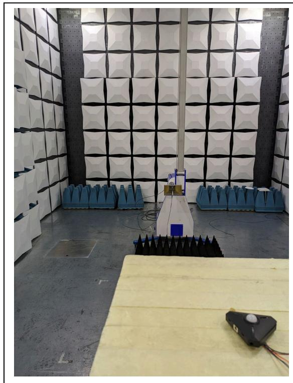
**Field Strength of Emissions: 18 GHz to 26 GHz, Occupied Bandwidth**
