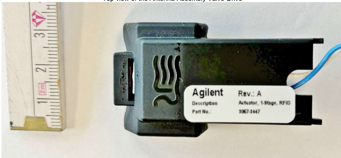
Top view of the Antenna-Assembly Valve-Drive
